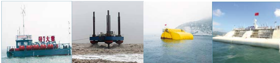
Figure 3.8: Prototypes of the wave energy converters tested in China (from left, 10kW Jida I (Wang et al., 2012); 10kW three-buoy WEC (Xia et al., 2014); 100kW DUCK III (Yao et al., 2016); 100kW Sharp Eagle Wanshan (Sheng et al., 2015a))
