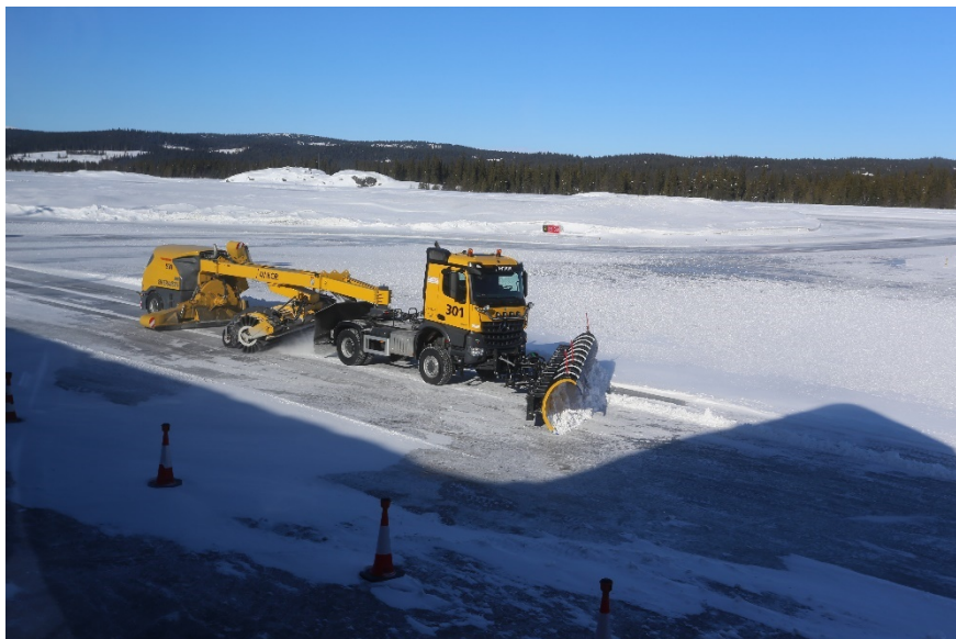
Figure 6: Test of Autonomous Plow Trucks at Fagernes Airport March 19, 2018. Credit: Avinor
