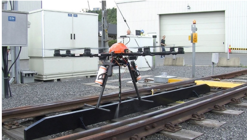
Figure 4: UAS used for Lubrication of Railroad Switches. Credit: Harry Korslund
