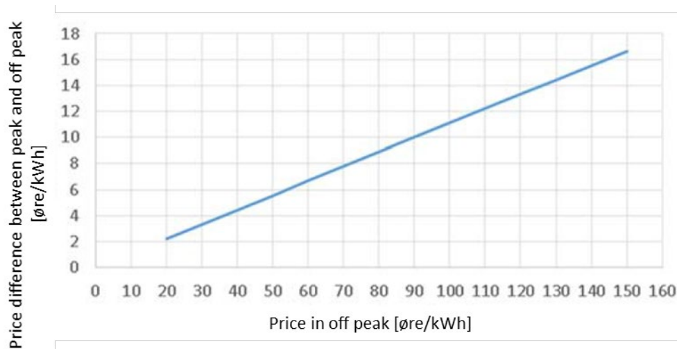
Figure 4.9 Necessary price differences to achieve an economical benefit from the use of battery [18]
