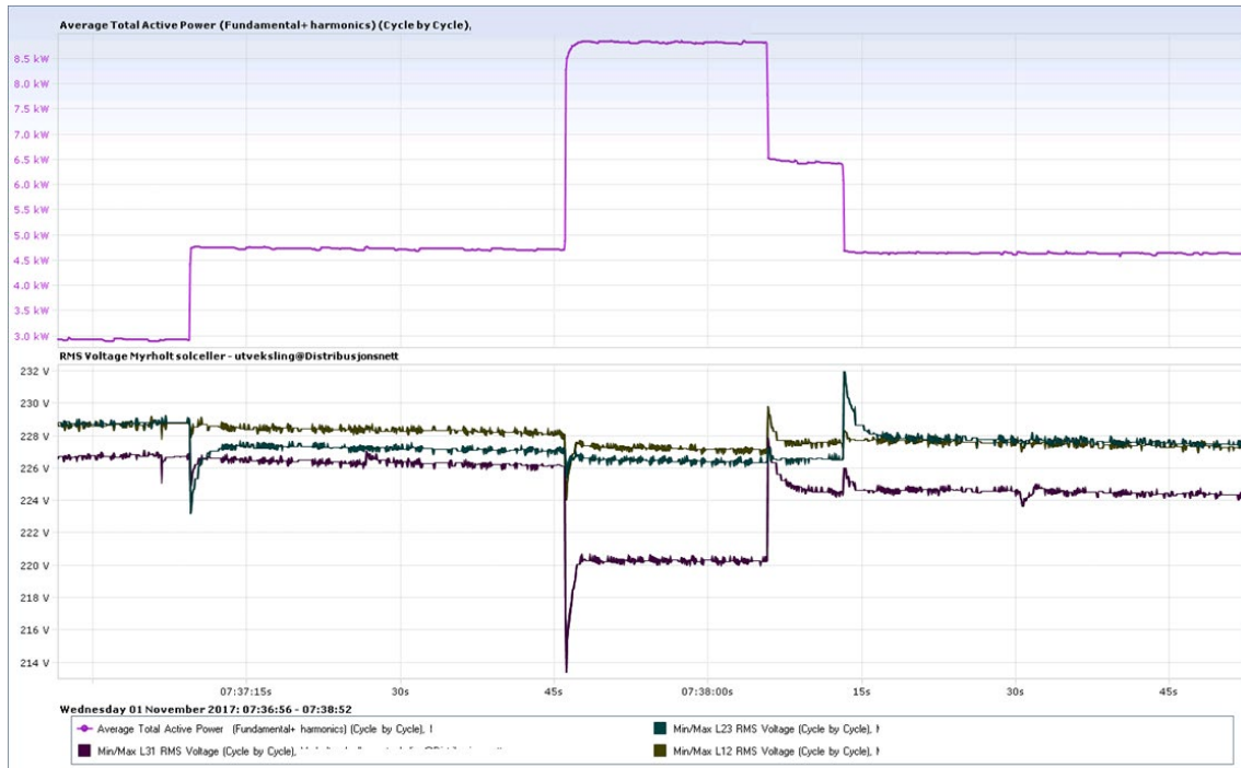
Figure 4.6 Meter data for 2 minutes, at the prosumer. Saturation (Source: NTE)
