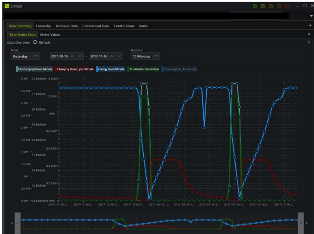
Figure 4.11 Interface showing State-of-Charge (SOC) for the battery (SOC curve - blue, discharging curve – light blue, charging profile – red, generation curve - green and consumption (not activated)) [5]
