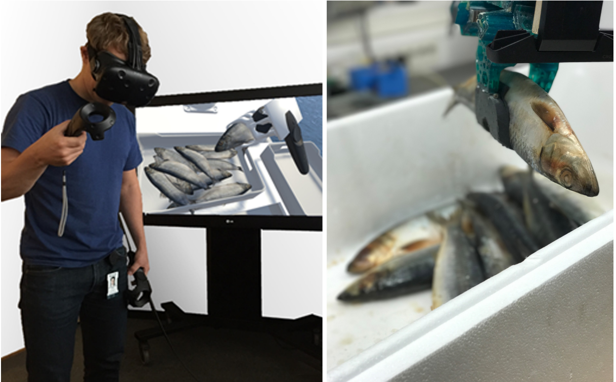
Figure 1: Teaching a robot to pick herring in virtual reality.
