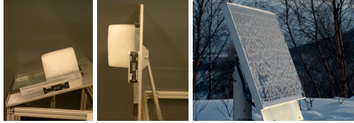
Figure 8: Snow/ice slab firmly sticking to the glass surface of an insulated window pane even at an inclination angle of 90° during a laboratory experiment (left). Snow covering a solar cell panel at an inclination angle of 70° (right) [21].
