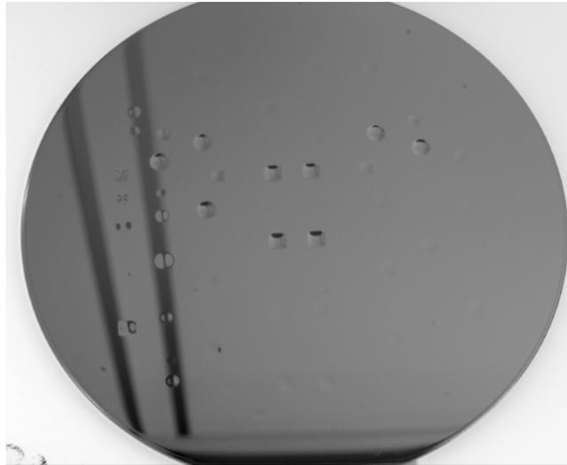
Figure 6. Picture of a 100 mm diameter wafer pre-bonded at 207mbar, after bond anneal. The membranes with visually clear deflection were found to show slip-lines similar to those seen on the vacuum reference wafer.
