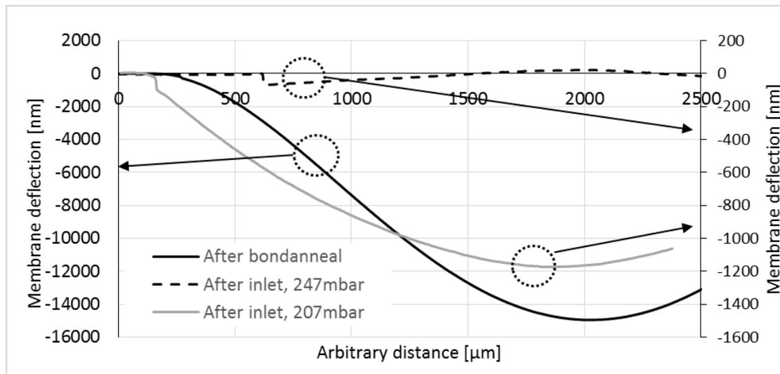
Figure 5. Profile plots from WLI measurements of C4-type membranes just after bond anneal and after INLET etch for 207 and 247 mbar. Please note the difference in scale. After INLET etch the membrane location has been made visible by the step created in the Si before bonding, but note that this step does not coincide precisely with the membrane edge.
