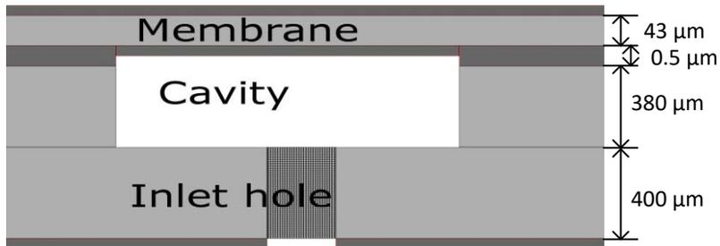
Figure 1. Sketch of test structure cross-section (not to scale). The inlet hole is etched by DRIE after bond anneal.
