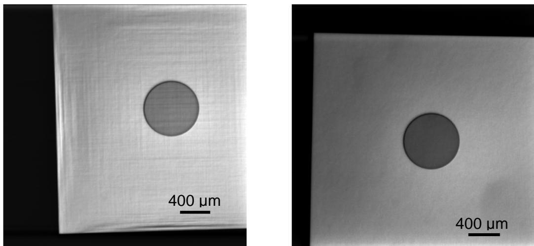
Figure 3. IR microscope picture of S4-type membranes pre-bonded in vacuum (left) and at 207 mbar (right). The light gray area is the membrane. The straight lines seen in the left hand membrane are slip-lines in the Si crystal. The dark circle is the oxide mask opening for inlet DRIE. Bar indicates  $400 \mu\text{m}$  length.
