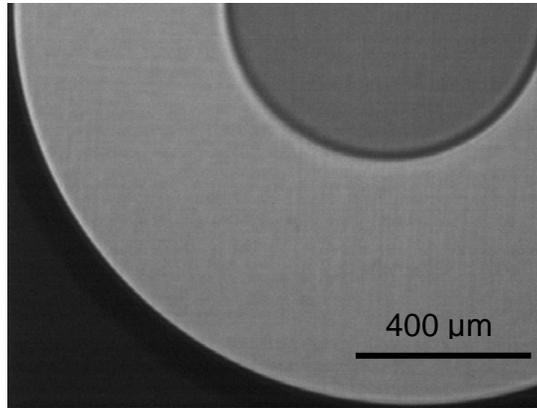
Figure 4. IR microscope picture of parts of a C2 membrane pre-bonded in vacuum. It is worth noting that there are slip-lines all over the membrane. Bar indicates 400  $\mu\text{m}$  length.
