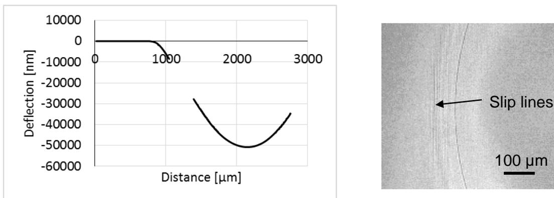
Figure 2. WLI measurement of a C3 type membrane pre-bonded in vacuum, after bond anneal (left). The break in the otherwise solid line appears because the wide angle of reflected light cannot be picked up by the WLI microscope. The right-hand picture shows the fringe mode picture from the WLI, with visible slip lines. Bar in lower right corner indicates  $100\ \mu\text{m}$  length.
