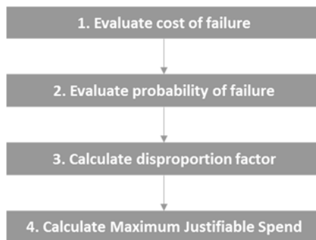
Figure 5: Flowchart of CBA based on the disproportion factor. Source: Paltrinieri and Khan (2016)
