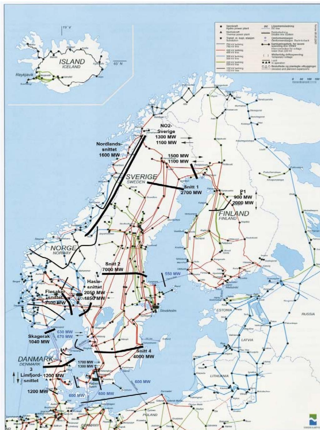
Figure 6 The transmission system in the Nordic region with relevant transmission constraints [5].
