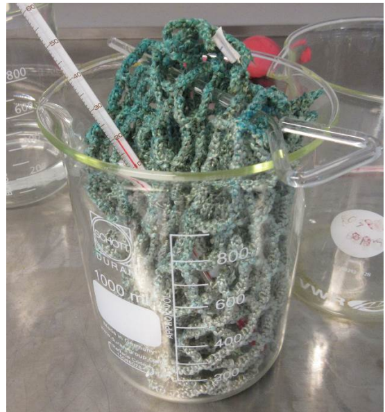
Figure A-4: Used netting with copper residuals, N 2 , subjected to 10 % Aqua Des (left) and concentrated Aqua Des (right).
