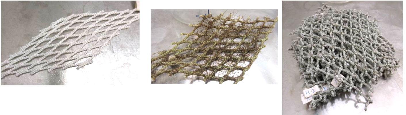
Figure A-1: Netting materials subjected to chemical exposure tests. From left: N1, N1_bf and N2.
