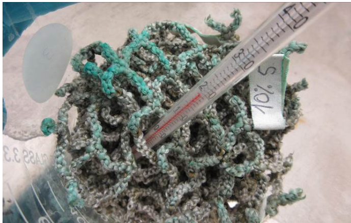
Figure A-4: Used netting with copper residuals, N 2 , subjected to 10 % Aqua Des (left) and concentrated Aqua Des (right).
