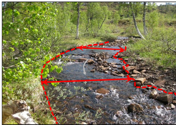
Figure 5-1: Wetted width for two transects of a river in the Norwegian mountains. The dashed lines indicate the water line along the shore for the actual flow conditions.
