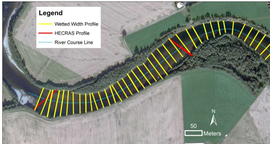
Figure 5-5: Example for extraction of wetted width transects for the Orkla river, Station 121.22, aerial image from 15 September 2009. From Zinke & Carnerero (2014).
