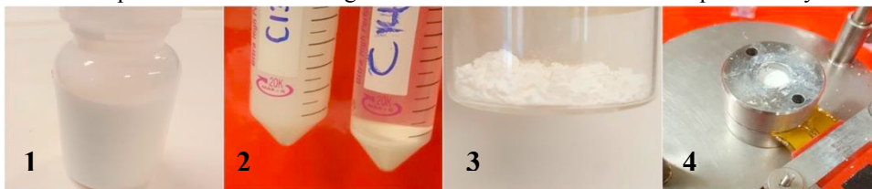
Figure 1: Results of the steps in the synthesis. The first and left photo shows the polystyrene templates produced (1), in the second photo the polystyrene spheres coated with silica particles are showed both before (left) and after (right) centrifuging (2), the third photo shows the dried silica spheres (3), and the fourth photo depicts the powder in the Hot Disk for measurement of thermal conductivity (4).
