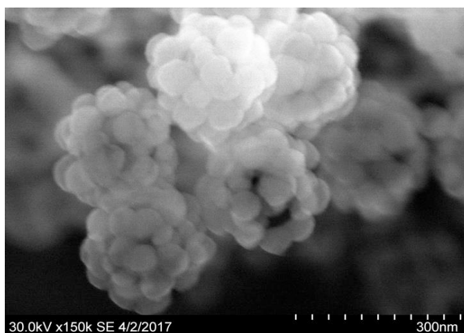
Figure 4: Scanning electron microscope (SEM) image of silica spheres produced by coating and drying of PS sample B.
