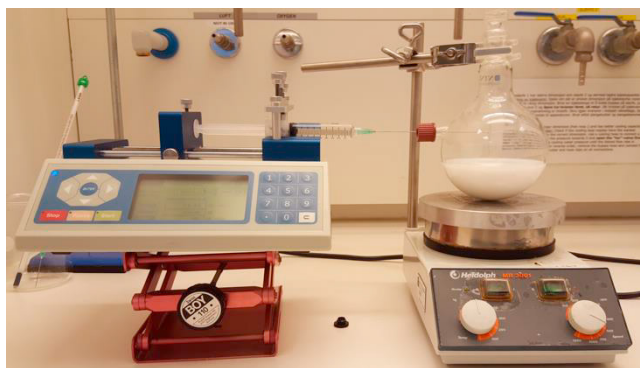
Figure 3: TEOS solution added dropwise to the round bottom flask with the use of a syringe pump, a 10 ml syringe and a horizontal opening in the flask.
