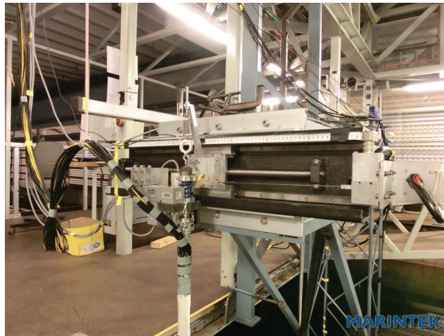
Fig. 4: Drilling riser top unit: One dof forced motion actuator, tensioner of marine riser, tensioner of drill string, heave compensation, UFJ, horizontal potentiometer and 3 component force measurement.
