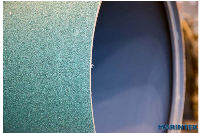
Figure 3 Rough surface modelled by sandpaper, k/D = 1.0 \times 10^{-3} .
