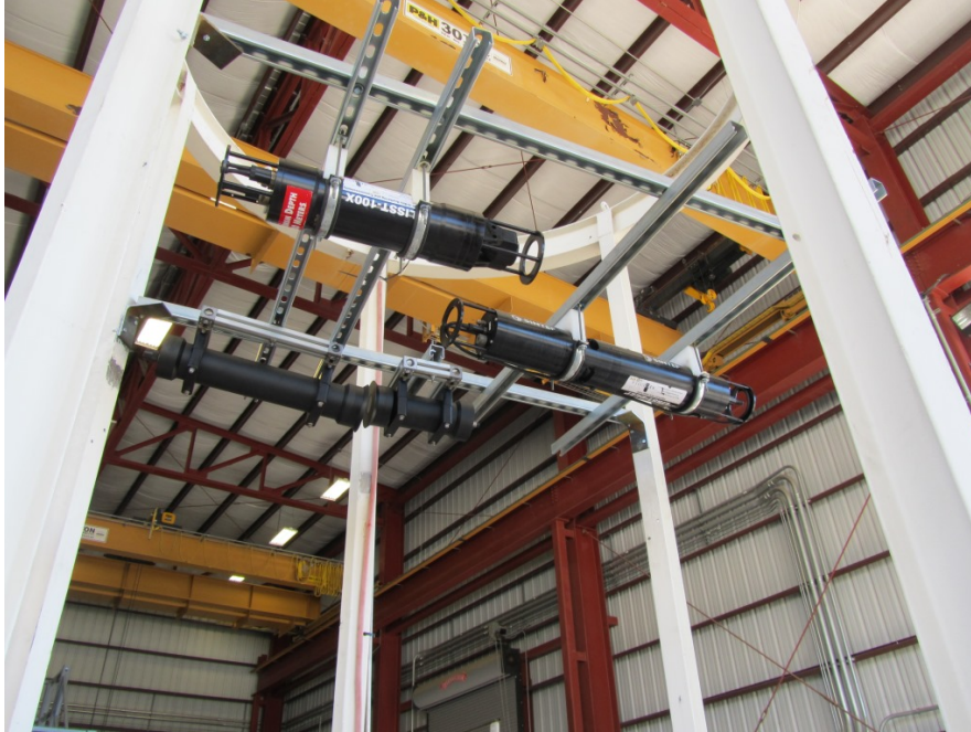
Figure A - 2: SINTEF Instruments Mounted to Test Frame
