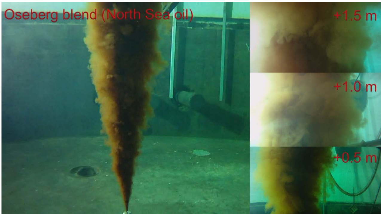
Figure A.7: An example of a composite video showing the four HD cameras covering the rising oil flume at 0.5 m intervals over the release point. This is from earlier experiments with a North Sea crude (Oseberg blend).
