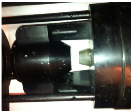
Figure A - 6: The path reduction module of the LISST-100X (round/conical prism). The LISST-100X and LISST DEEP were used during the initial testing (see Appendix C for details).
