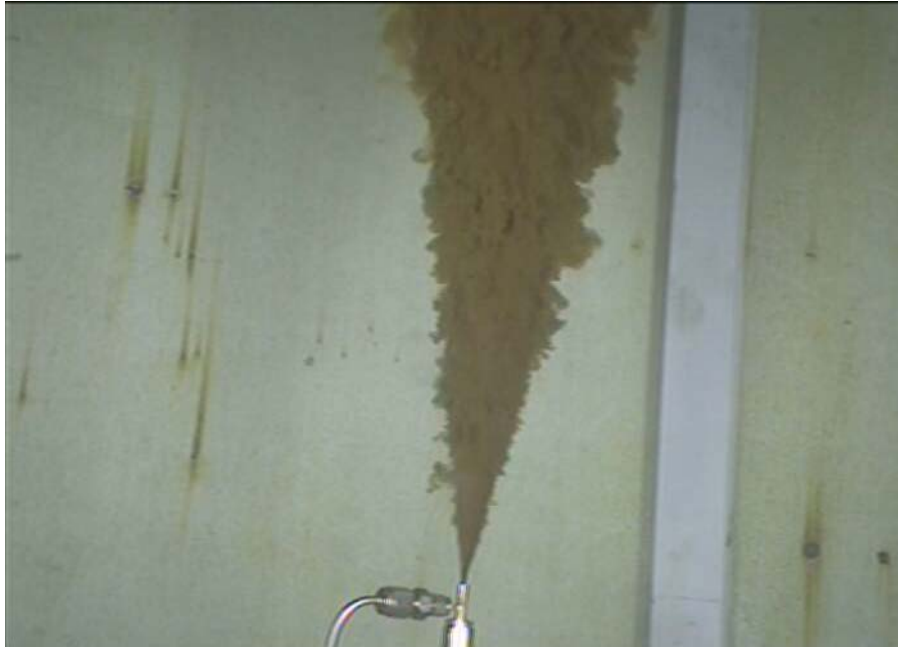
Figure A - 3: Screen Capture of Video during High Pressure Test, Dispersant Introduced (1% C9500)
