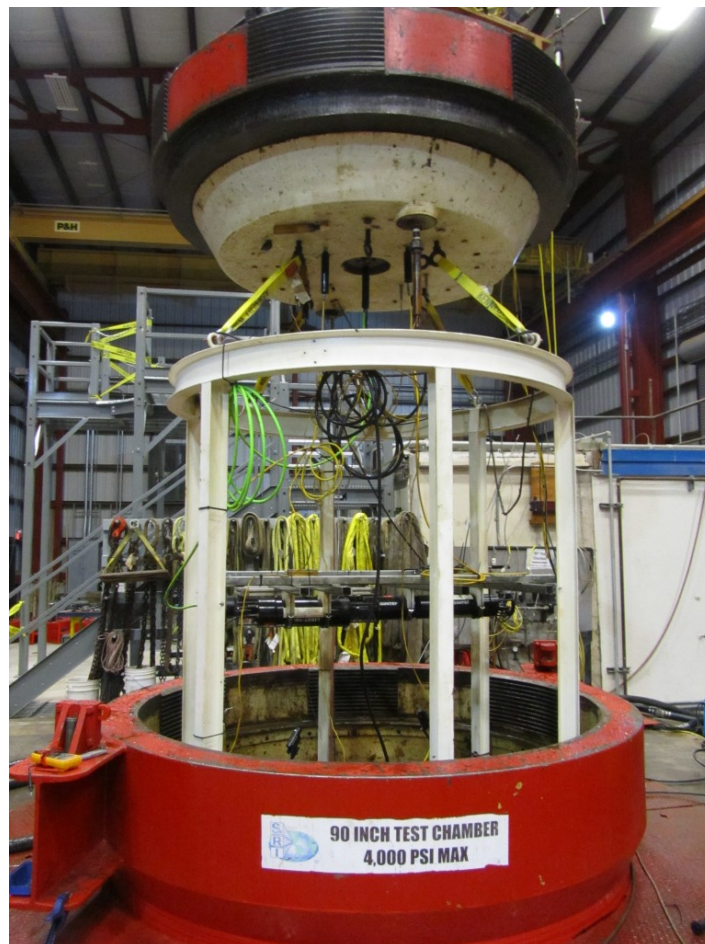
Figure A - 4: Chamber Ready for Test Prior to Frame Install
