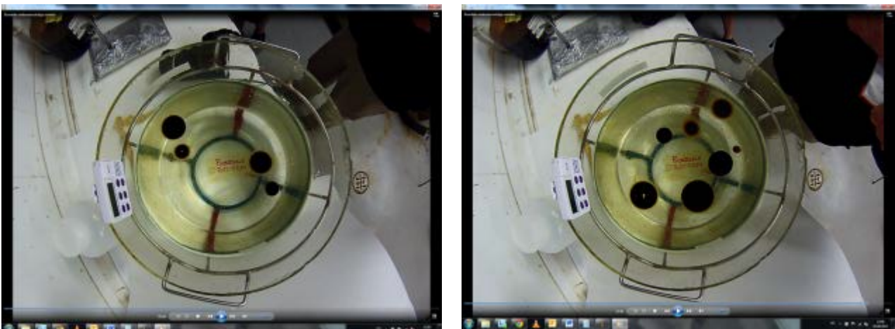
Figure 3.18 RFA Boardale; subsurface release. First application (left) 10 oil droplets and second application (right) with a total of 50 oil droplets.
