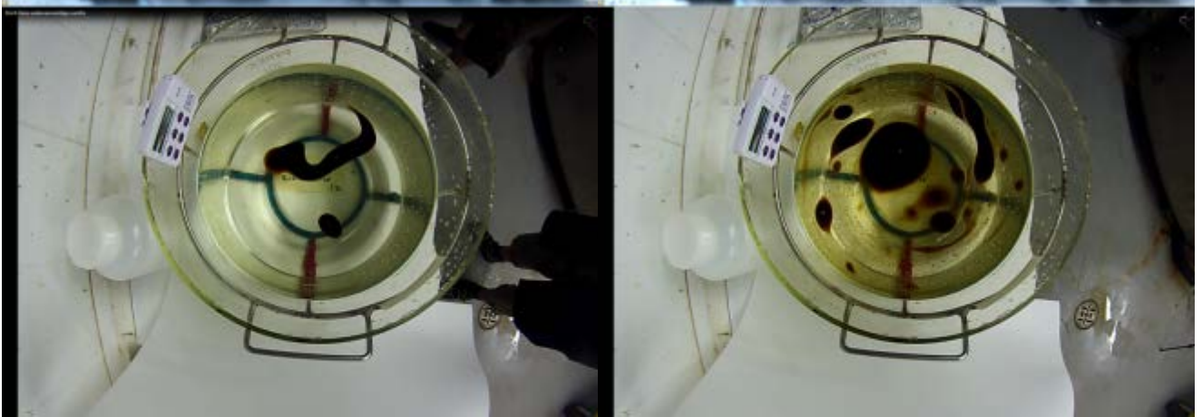
Figure 3.16 Erich Giese; subsurface release. First application (left) 10 oil droplets and second application (right) with a total of 50 oil droplets.
