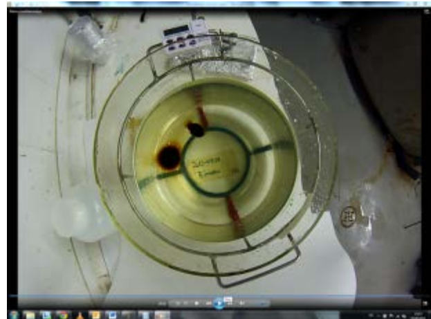
Figure 3.14 HMS Bittern; surface release. First application (left) 10 oil droplets and second application (right) with a total of 50 oil droplets.
