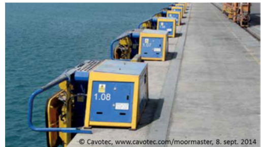
Figur 44: MoorMaster™ – vakuumbasert fortøyning
