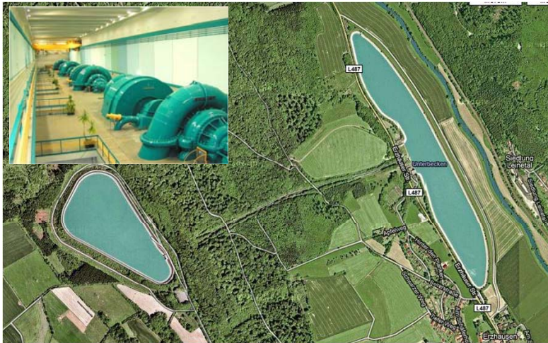
Statkraft 220 MW turbines/pumps, 1035 MWh storage
