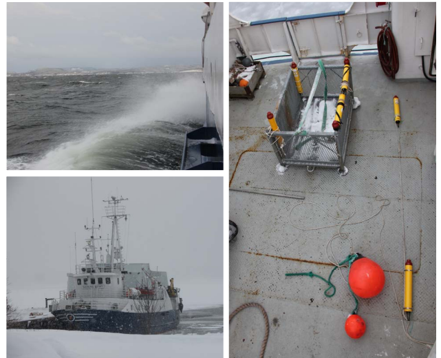
Figure 10. Modem range test scenario and equipment including all 6 UAN modems
