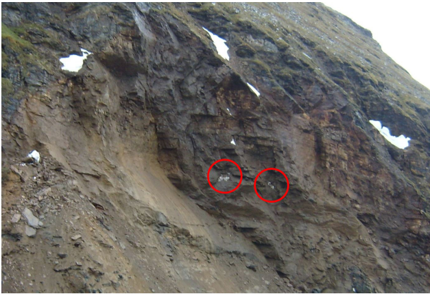
Figure 2. Visible in situ ice (encircled areas) observed in the rock avalanche failure zone on 26 June 2008. The photograph was taken a few hours after the event (Photograph by courtesy of Kjetil Bratlien, NGI).
