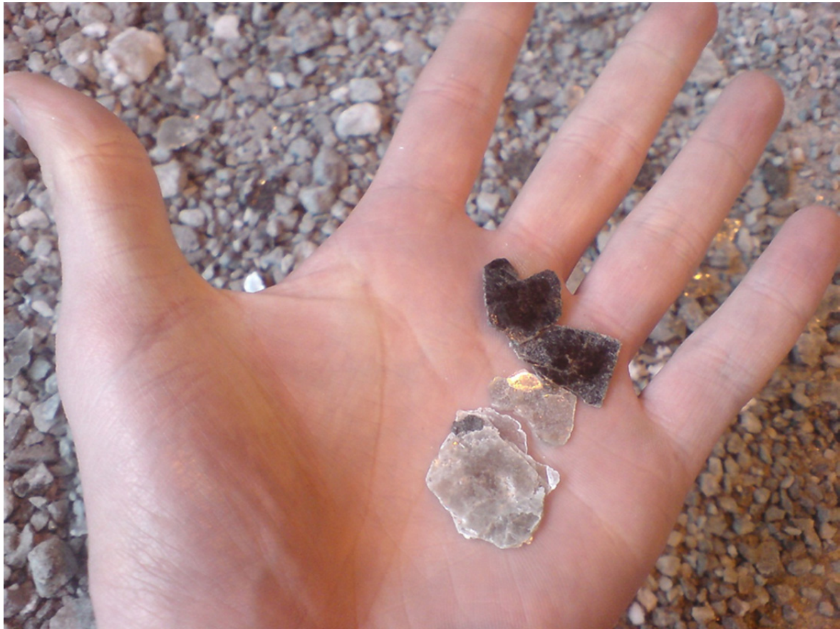
Fig. 2-3: Flaky mica particles in oversize feed material 22/40 mm from Hokksund Pukkverk AS (Cepuritis 2011)
