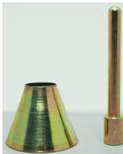
Fig. 2-4: Truncated steel cone and tamper that are used according to EN 1097-6 (2002) in order to assess if a sand sample has reached the SSD state (UTEST 2012)
