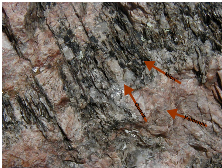
Fig. 2-1: Rock types of the fillers used for the study: granite (source: unknown)
