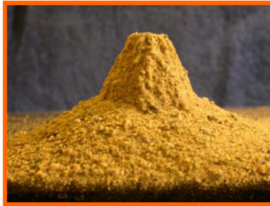
Fig. 2-7: Aggregate SSD; the cone shape has just collapsed; the height is reduced for about 0.5-1 cm due to tamping with the steel tamper (NBTL 2003)
