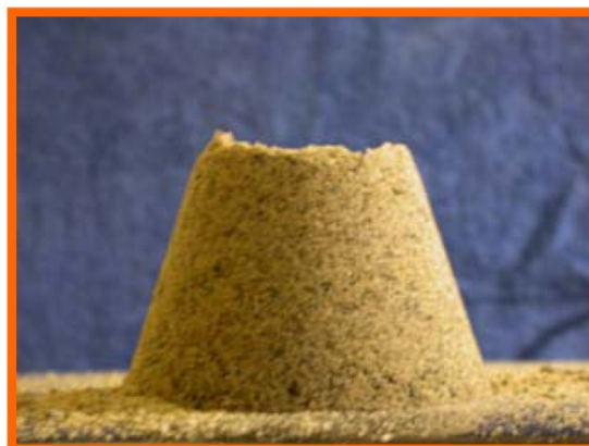
Fig. 2-6: Aggregate moist; complete shape of the metal moulds; the height is reduced for about 2-3 cm due to tamping with the steel tamper (NBTL 2003)
