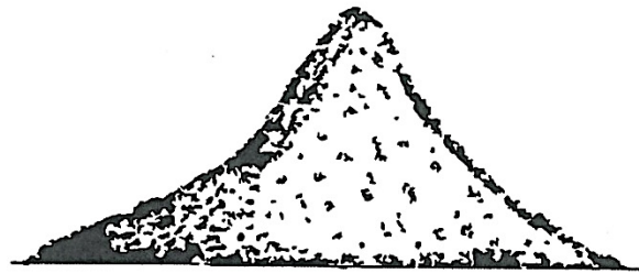
b) Aggregate slightly moist; appreciable slump observed
