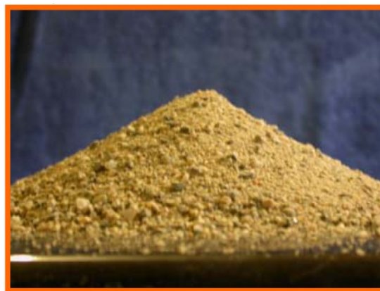
Fig. 2-8: Aggregate dry; the cone shape has totally collapsed and slopes are angular – a “new cone” with a clear peak has occurred; the aggregate has been oven dried for 24 hours at 105 °C (NBTL 2003)
