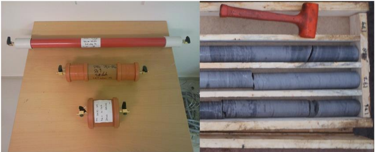
203 Fig. 2: Drilled cores from the wells on the right and custom-built cylindrical 204 polyethylene containers for core degassing on the left
