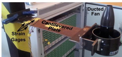
**Figure 5.** Fan Set Up for Calibration
