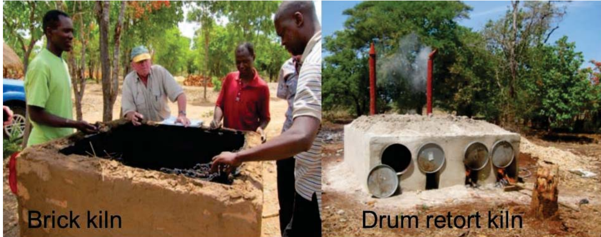
Fig. 1. Brick and drum retort kiln used in the production of BC used in field experiments. Photos taken by G. Cornelissen.
