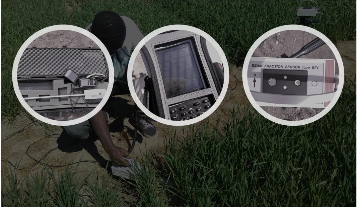
Figure 3.3 Measuring light transmission with a Sun scan comprising of a probe(left), PDA (centre), and (BFS1) right
