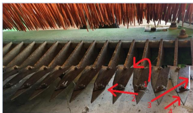
Figure 1 Knife bar of the CombCut. 1: Vertical angle adjustment to increase opening between knives. 2: Horizontal angle adjustment to force leaves towards blade. 3: blade. 4: blade holder
