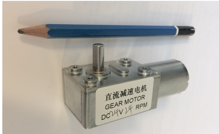
Figure 5.2: 24 V DC motor with worm drive.
