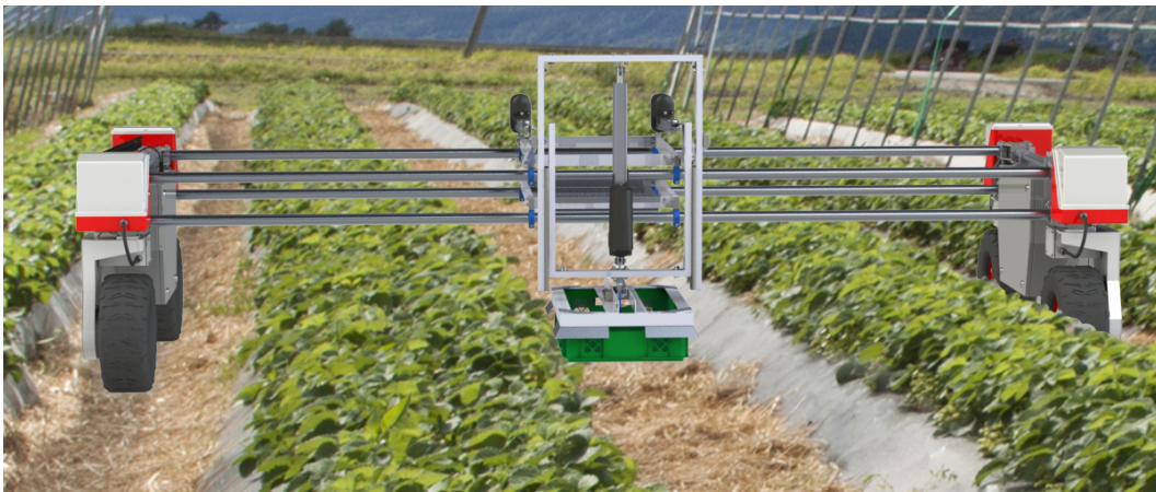
Figure 6.14: Photo manipulation of the robot platform in a double-row environment.
