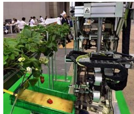
(d) The green house based picking robot Berry Nice [29]
