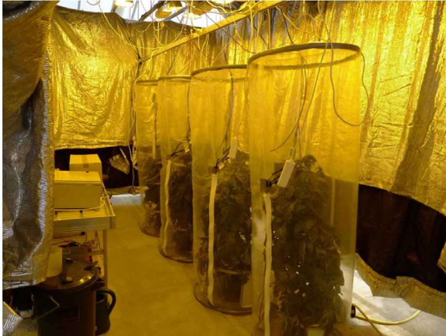
Figure 3.1. Gas exchange chambers with tomato plants (Further described in paper 4). Air entered the chamber from an inlet at the base and left at the top. Climate parameters were measured at plant level.
