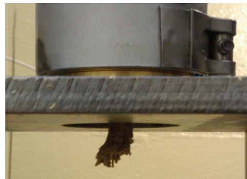
Figure 6. Flow of Pine Scots through the laboratory die pelleting rig
