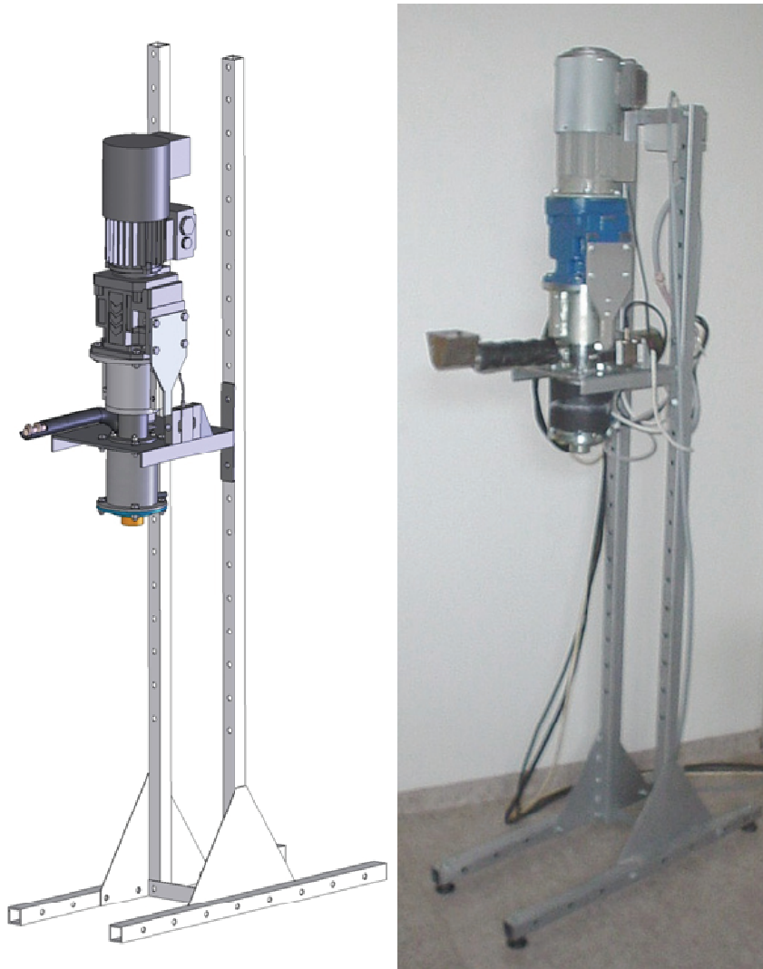
Figure 15: At the left the 3D model of prototype I and at the right the built prototype I (without recirculation path).
