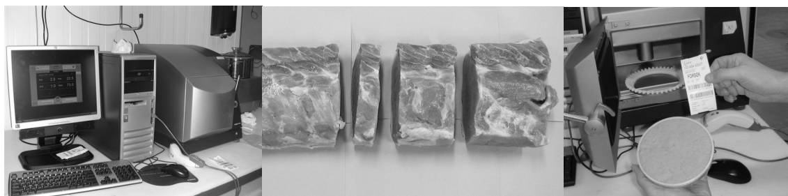
Figure 8 - (1) The FOSS FoodScan near-infrared spectrophotometer (FOSS, Denmark) used for the determination of fat, moisture and protein in (2) the LD muscle. (3) Approximately 180 g of ground samples were placed in a 140mm round sample dish, and the dish was placed in the NIRS instrument. A barcode was used for identification purposes. Photos: Gjerlaug-Enger and Kringberg.
