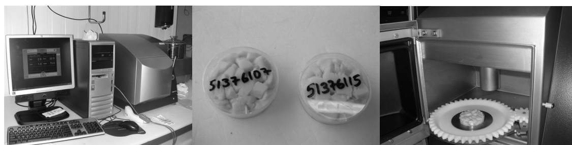
Figure 9 - (1 and 3) The FoodScan near-infrared spectrophotometer (FOSS, Denmark) was used to determine the fat moisture content in (2) subcutaneous fat samples. Photos: Gjerlaug-Enger.
