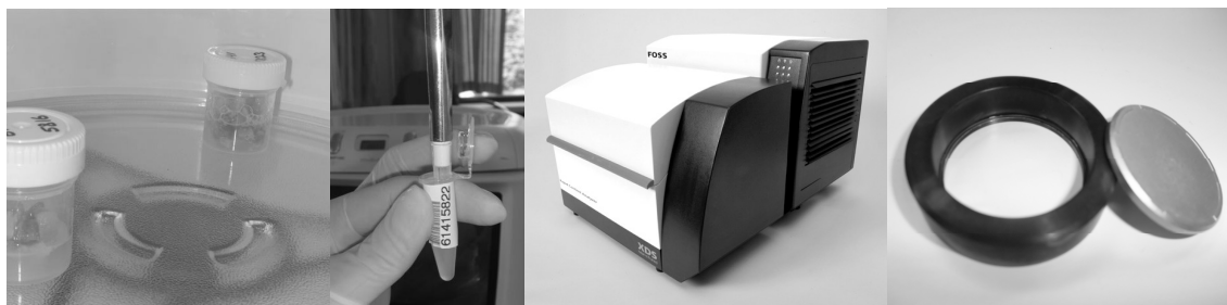
Figure 10 - (1) A microwave fat melting technique was used for the samples preparation. (2) Total lipid was added to Eppendorf tubes with a pipette. (3) The XDS near-infrared rapid content analyser. (4) Scanned once using a circular quartz cuvette and a gold plated reflector provides optical path lengths of 0.2 mm. Photos: (1, 2, 4) Gjerlaug-Enger, (3) www.foss.com .
