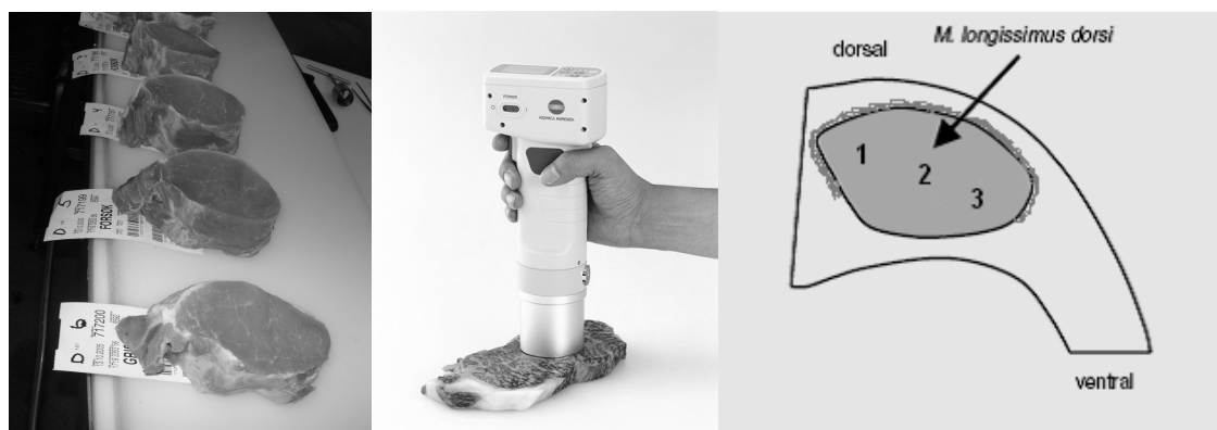
Figure 7 - The meat colour was measured using (2) a Minolta Chroma Meter CR-400 on (1) bloomed chops of LD muscles. (3) Measuring positions, with duplicate measurement in three positions.
