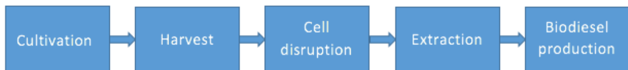
Figure 2.1: Outline of the microalgal biodiesel production process
