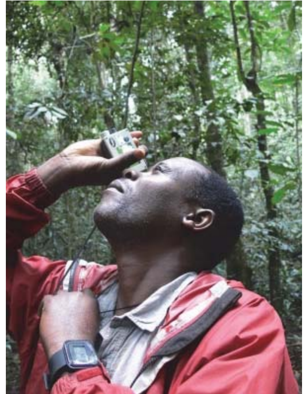
Figure 5. Measuring tree height using a Vertex IV hypsometer.
