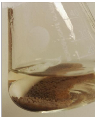
Figure 43: Dried Amberlyst-16w right after addition of ethanol 96% to the beaker
