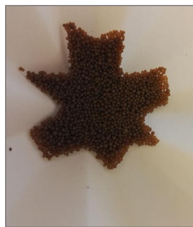
Figure 39: Remaining Amberlyst -16w after filtering out the liquid
