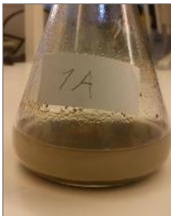
Figure 32: T-6812 after stirring with magnetic stirrer in rectified ethanol for 120min, T=ambient
