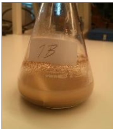
Figure 28: T-63 and 96% ethanol after 120 minutes stirring, T=ambient
