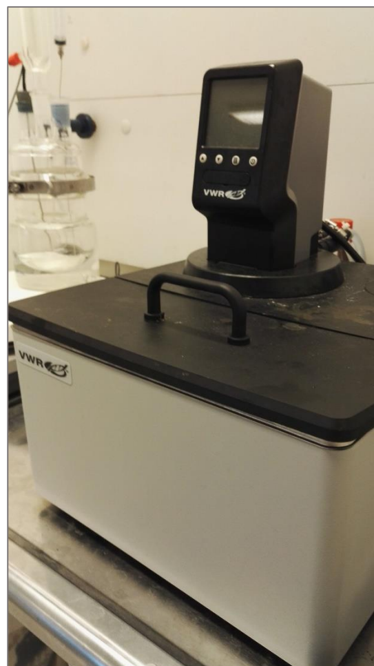
Figure 25: The warm water bath, heating water to a given temperature and sending it through the outer container to heat the content of the inner.
