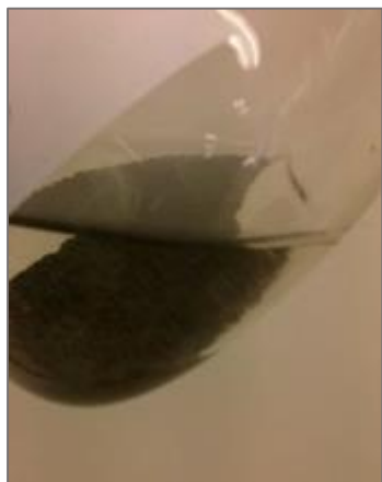
Figure 31: T-6812 initially after addition of rectified ethanol to the untreated catalyst, T=ambient
