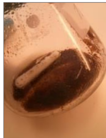
Figure 33: T-6812 remaining after 120minutes of reaction with rectified ethanol
