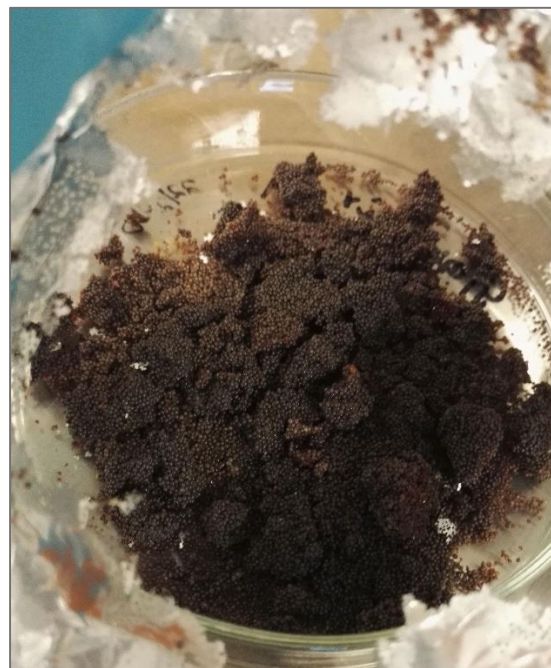
Figure 35: T-6812 used in reaction with absolute ethanol, which has laid over a week on aluminium foil, corroding through the foil.
