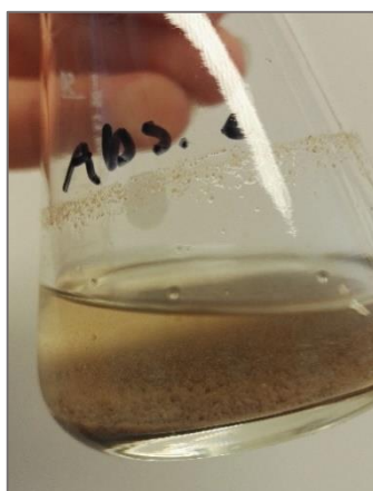
Figure 41: Dried catalyst and absolute ethanol after 120 minutes stirring in the beaker
