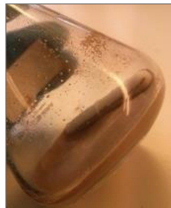
Figure 29: T-63 remains after 120minutes stirring in 96% ethanol
