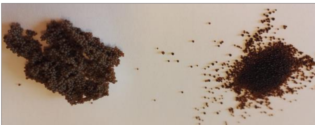
Figure 48: A picture of the catalyst straight from the container is shown to the left, to the right is the untreated catalyst after air exposure for over three days.
