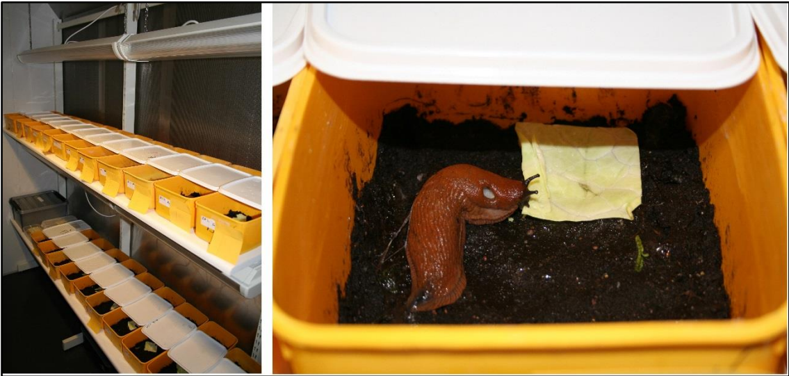
Figure 3: Left: The bioassay setup with 45 half covered plastic boxes. Right: An A. vulgaris in its arena, feeding on a cabbage square (4 x 4 cm).
