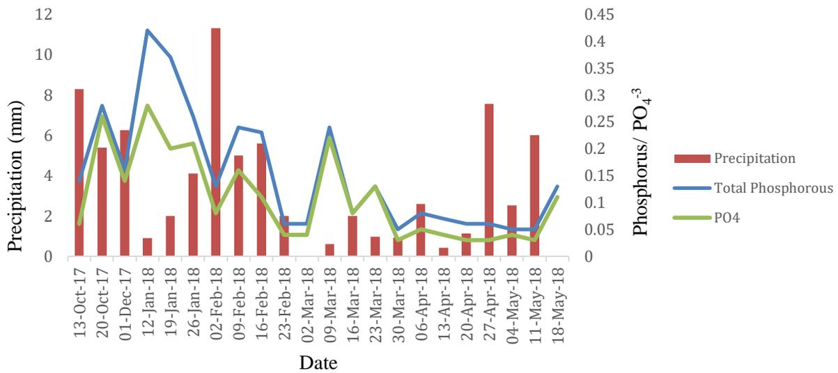
Figure 4-3 Total phosphorus and phosphate (PO<sub>4</sub><sup>-3</sup>) in Madlabekken stream together with precipitation
