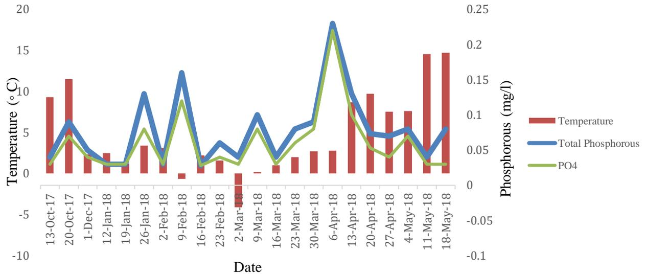
Figure 4-10 Total phosphorus and PO<sub>4</sub><sup>3-</sup> concentrations of Madlabekken wetland at the outlet, with temperature during the study period
