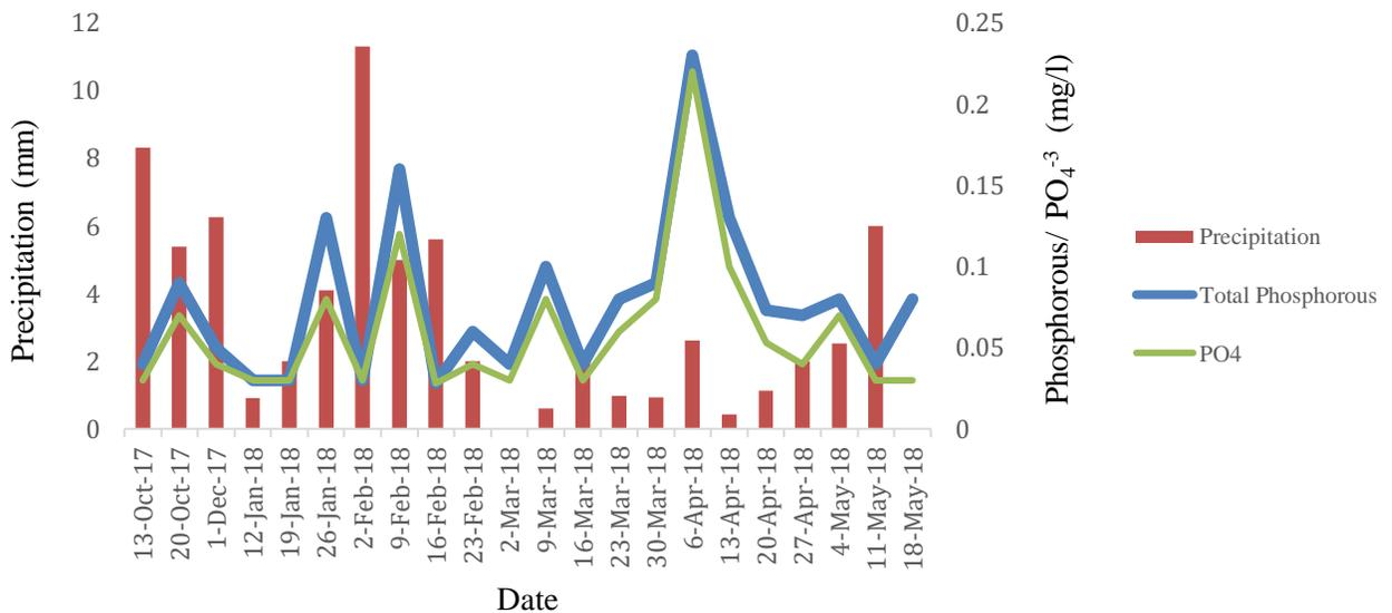
Figure 4-9 Total phosphorus and PO<sub>4</sub><sup>3-</sup> concentrations of Madlabekken wetland at the outlet, with precipitation during the study period
