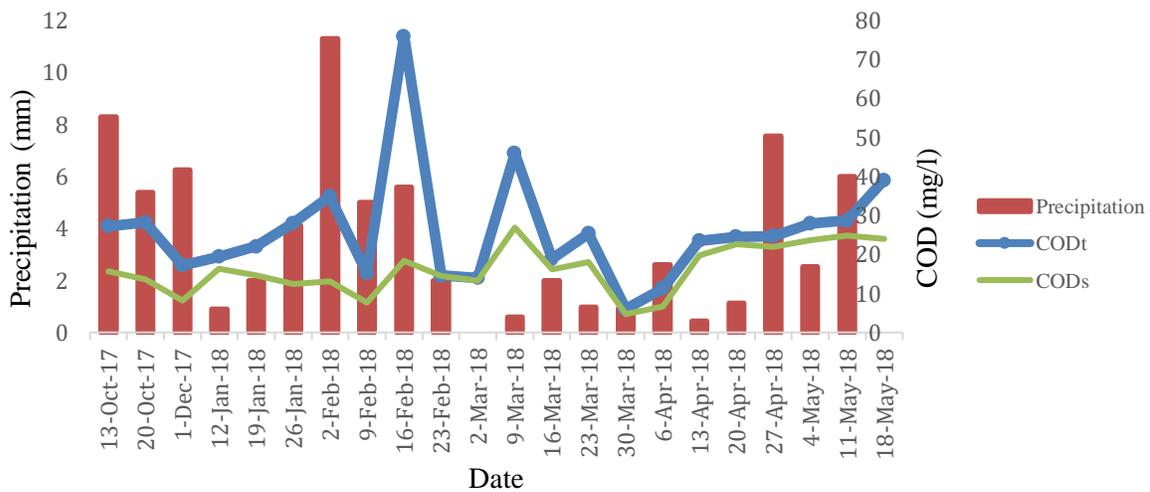
Figure 4-2 Total COD and soluble COD in Madlabekken stream at the inlet of wetland with precipitation
