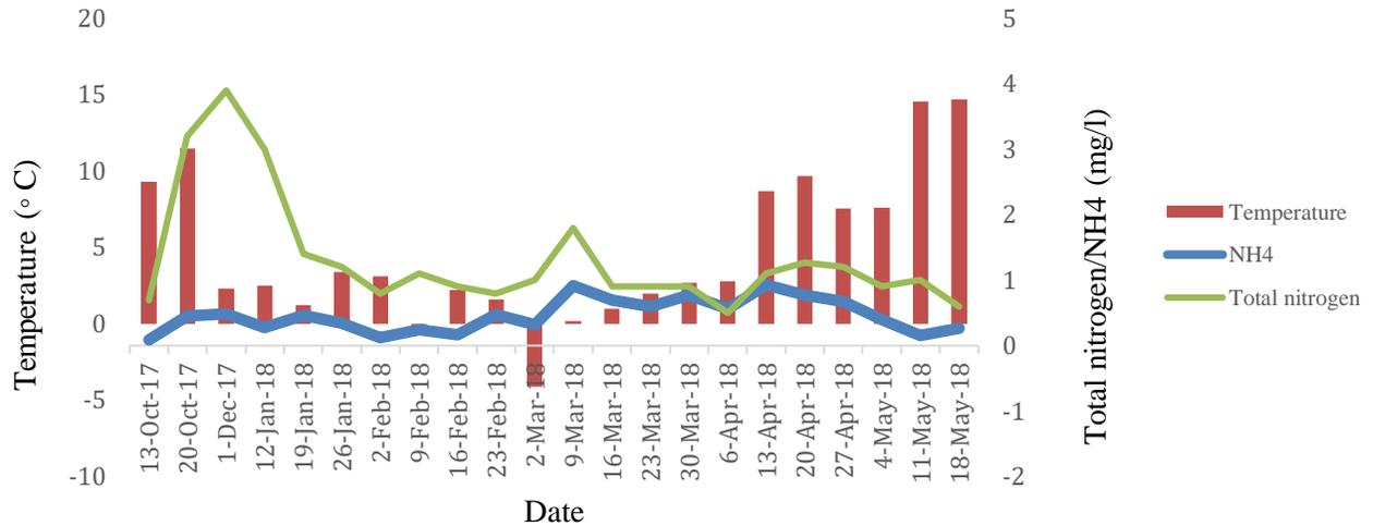
Figure 4-12 Total nitrogen and  $\text{NH}_4^+$  concentrations of Madlabekken wetland at the outlet, with temperature during the study period
