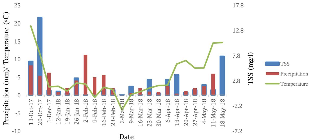
Figure 4-7 Total suspended solids of Madlabekken wetland outlet with precipitation and temperature during the study period
