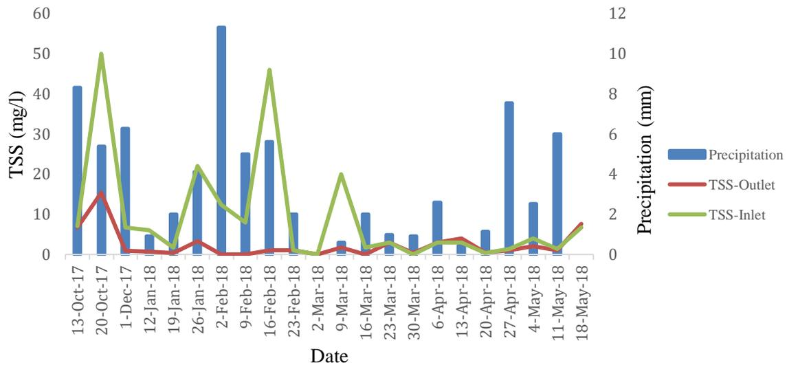
Figure 4-13 Total suspended solids from Madlabekken wetland inlet vs. outlet, October to May
