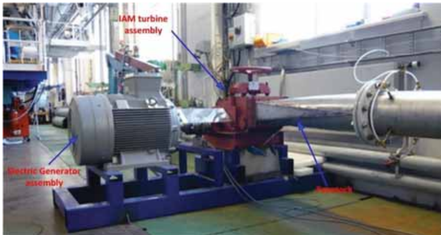
Figure 2.10. Experimental setup for IAM turbine at NTNU [3]
