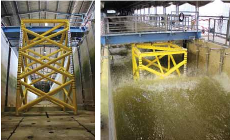
Figure 2.2 Wave Slam experimental set-up
