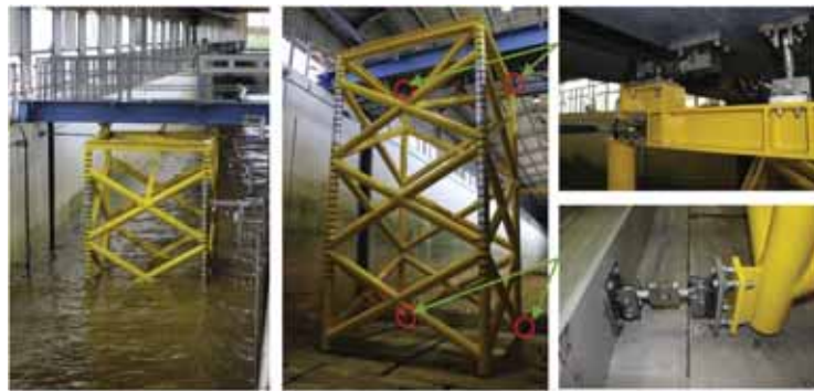
Fig. 2. Instrumented jacket structure in the wave tank. Total force transducers are marked by red circles.
