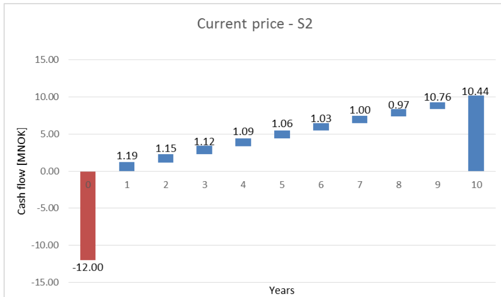
Figure 44: The cash flow for scenario 2 with the current fuel price and a return rate of 3%.
