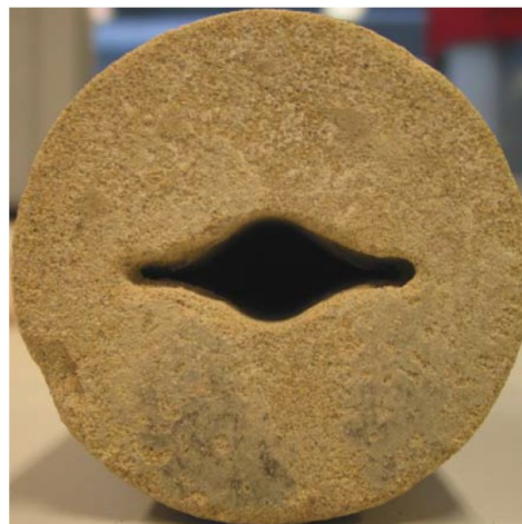
Figure 5 Production cavity after sand production, [4] figure 9
