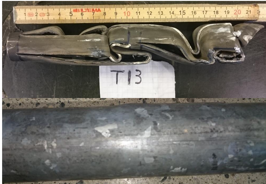
Fig. 67. The top picture shows specimen T13 after loading and ejection from the constraining tube. The bottom picture shows deformation of the constraining tube, as seen after the second test run.
