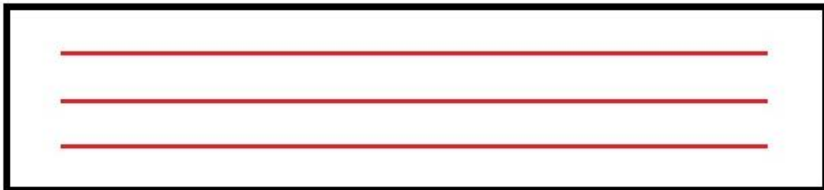
Fig. 42. Cutting pattern of specimen T7, where the uncut ends were approximately 10 mm long and the cuts were around 380 mm long.
