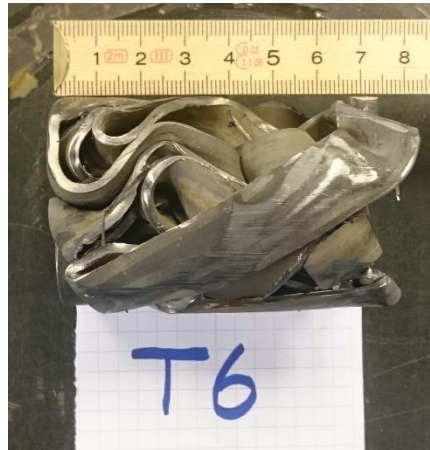
Fig. 41. Specimen T6 after crushing and ejection from the constraining tube.
