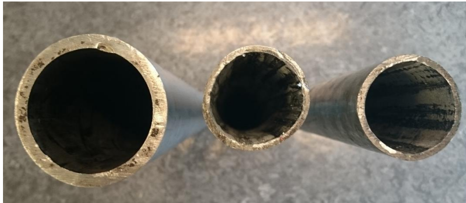
Fig. 32. The two different constraining steel tubes, the one on the left with an ID of 49.3 mm and the two others with an ID of 36.8 mm. The picture was taken after the experiment was finished, which is why the middle tube is deformed.
