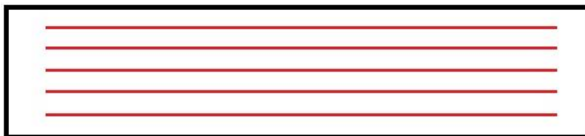
Fig. 39. Cutting pattern of specimen T6, where the uncut ends were roughly 10 mm long and the cuts were around 380 mm long.
