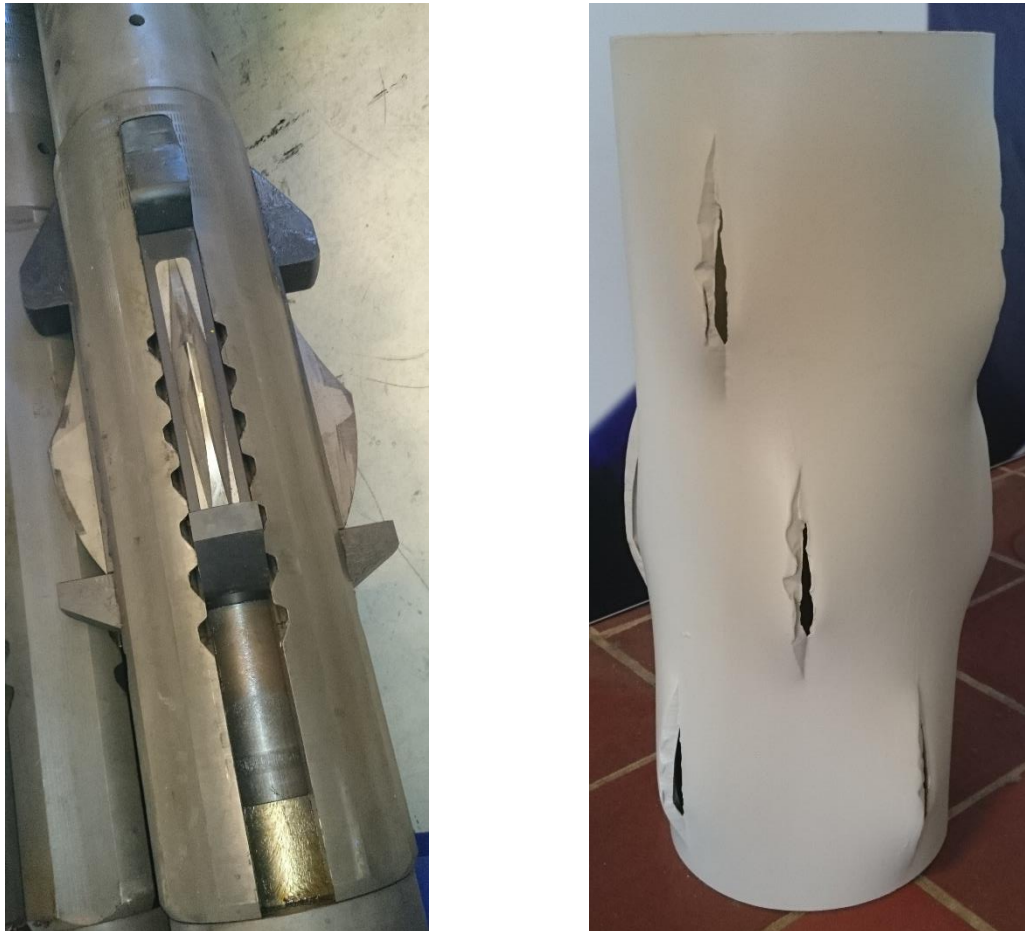
Fig. 89. To the left, a Gator Perforator tool designed by Lee Energy Systems Inc. To The right, a casting of a casing after being subjected to the Gator Perforator.
