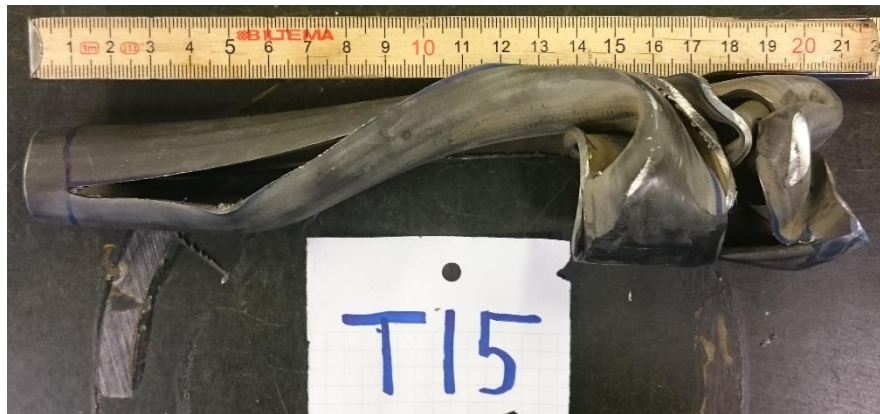
Fig. 75. Specimen T15 after loading and ejection from the constraining tube.
