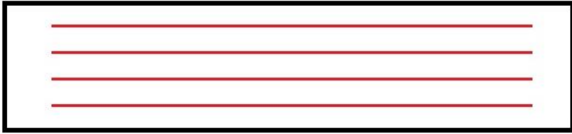
Fig. 50. Cutting pattern of specimen T9. This specimen was similar to T5, but placed within a larger constraining tubular for comparison purposes. The uncut ends were around 10 mm long, and the cuts were roughly 380 mm long.
