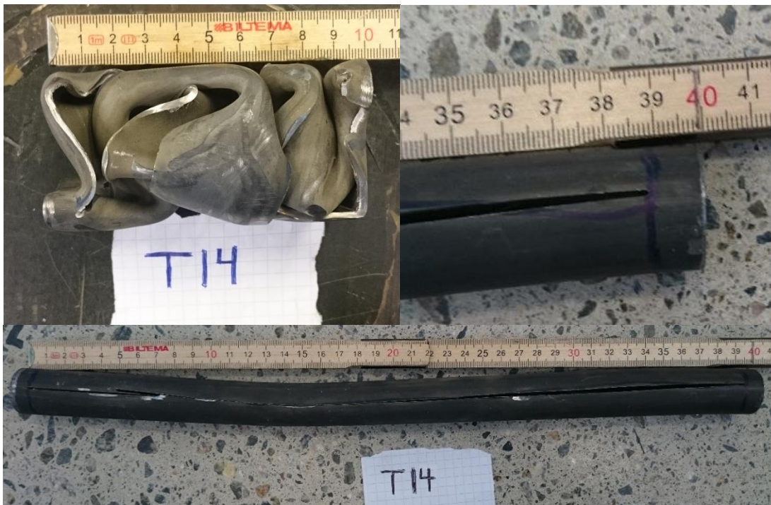
Fig. 71. The upper-left picture shows specimen T14 after loading and ejection from the constraining tube. The bottom picture shows the specimen after the first test run, while the upper-right picture shows the insignificant strain after this test run.
