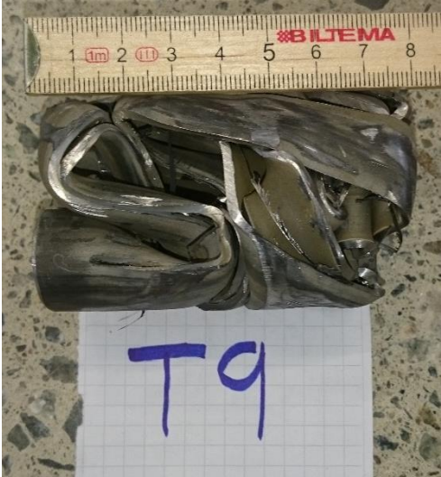
Fig. 52. Specimen T9 after loading and ejection from the constraining tube.
