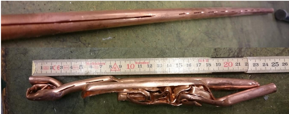
Fig. 93. The upper picture shows specimen T2 after cutting and before compaction. The lower picture shows the tube after crushing, and in this picture, the left side of the specimen was at the top, unlike all the other figures.
