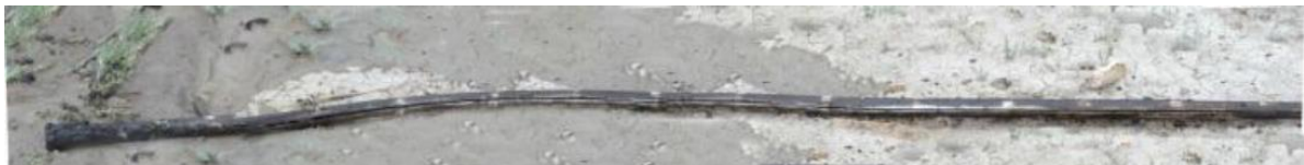
Fig. 16. The tubing was helically buckled and plastically deformed (Oilfield Innovations 2013).
