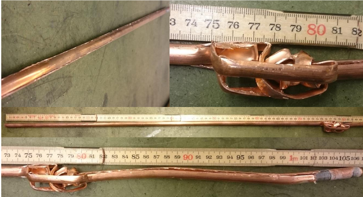
Fig. 91. Top left picture shows specimen T1 after cutting and before compaction. Top right picture shows the 3-cut section after crushing, the second picture from the bottom shows the lower end of the specimen, and the bottom picture shows the upper section of the specimen.
