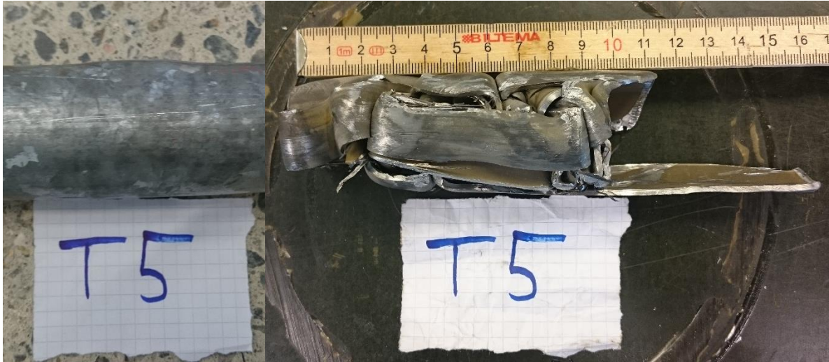
Fig. 37. To the left, the constraining tube is seen after the final test run. To the right, specimen T5 is pictured after crushing and ejection. Note the long metal piece extruding on the edge of the upper part of the crushed specimen.
