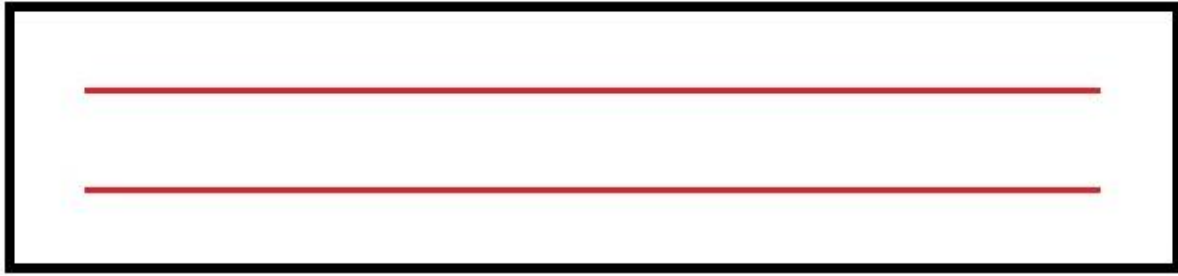
Fig. 69. Cutting pattern of specimen T14, where the uncut ends were around 10 mm long and the cuts were roughly 380 mm long.
