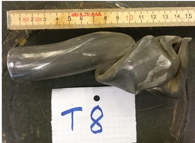
Fig. 48. Specimen T8 after loading and ejection from the constraining tube.
