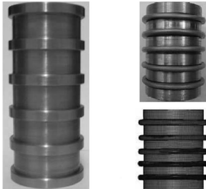
Fig. 7. To the left, a test specimen with wide external grooves before compaction. To the right, a specimen after compaction, from experiment at the top and from numerical simulation at the bottom (Salehghaffari, Tajdari and Mokhtarnezhad 2009).
