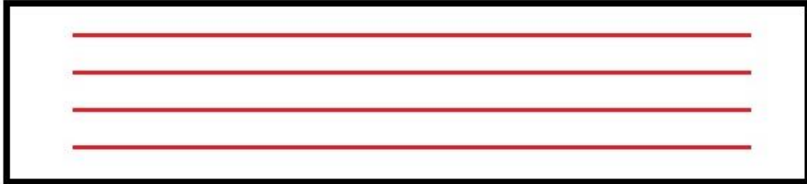
Fig. 35. Cutting of specimen T5, where the uncut parts at the ends were approximately 10 mm long. This means that the cuts were around 380 mm long.
