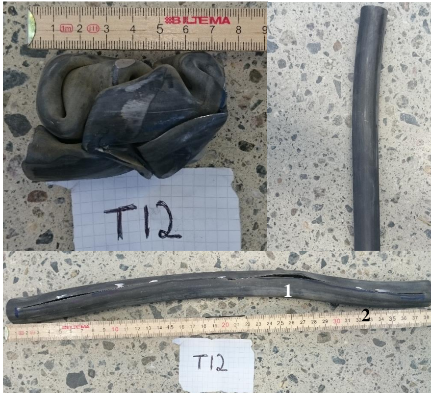
Fig. 63. The top-left picture shows specimen T12 after loading and ejection from the constraining tube. The top-right picture shows the bent test specimen after the first test run, and the bottom picture shows the buckled specimen after the second test run.
