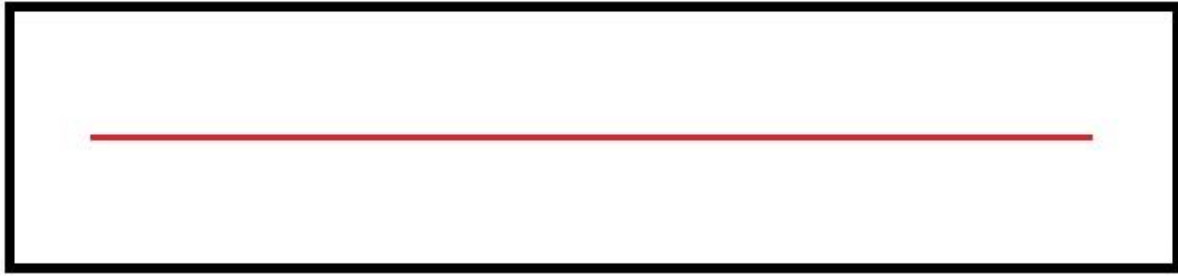
Fig. 61. Cutting pattern of specimen T12, where the uncut ends were around 10 mm long and the cut was roughly 380 mm long.
