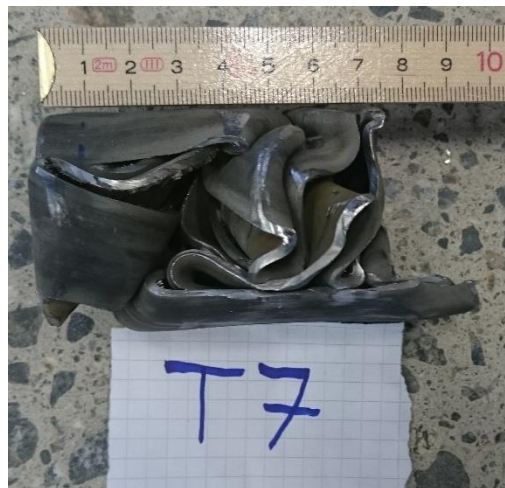
Fig. 44. Specimen T7 after crushing and ejection from the constraining tube.
