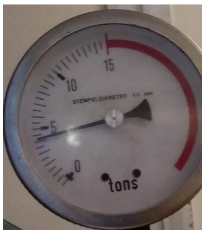
Fig. 38. Maximum frictional force during ejection of specimen T5 using the manual pumping press.
