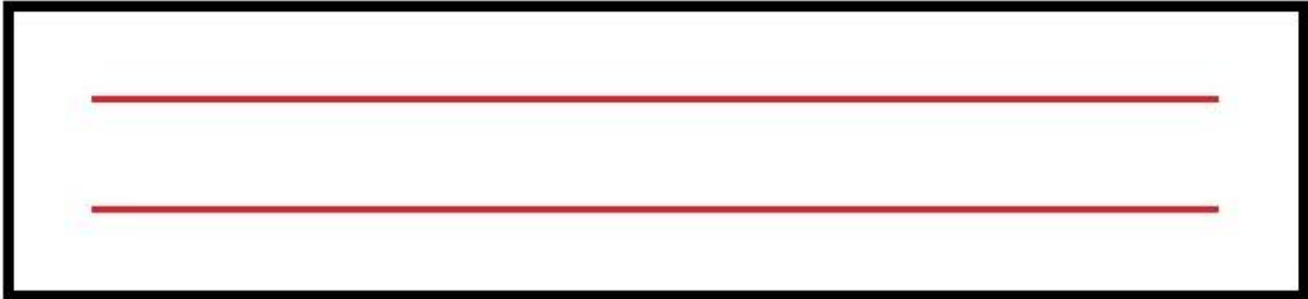
Fig. 73. Cutting pattern of specimen T15, which was aimed to be identical to that of specimen T14. The uncut ends had a length of around 10 mm and the cuts were roughly 380 mm long.
