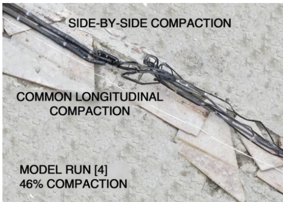
Fig. 19. The crushed tubing from model run [4] after ejection from the casing (Oilfield Innovations 2013).
