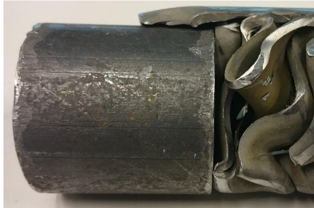
Fig. 85. The extension rods did not fill the entire internal area of the constraining tube. This caused metal pieces to extrude adjacent to the extension rod.
