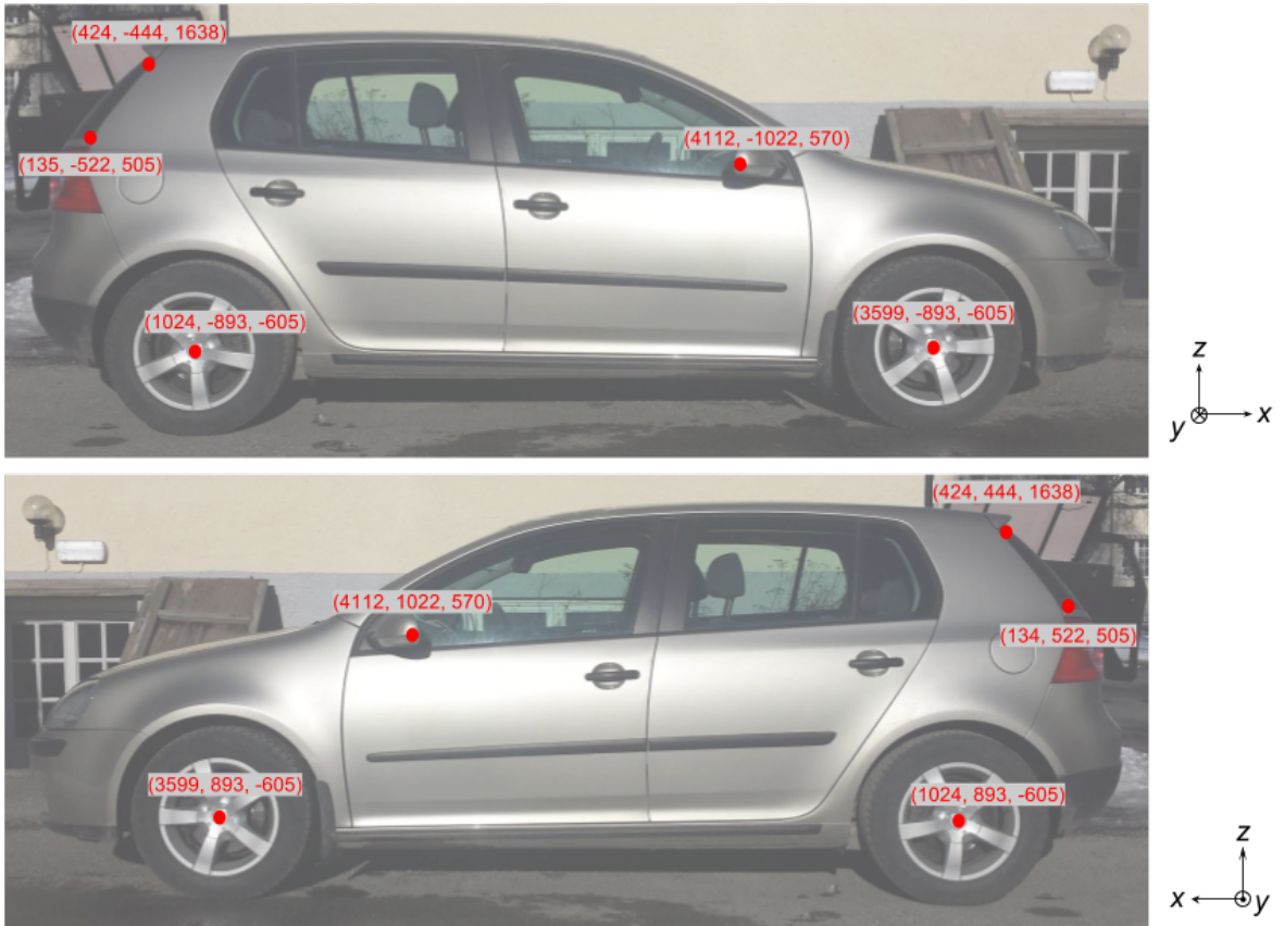
Figure 4.21: 3D model of the Golf. All feature points are relative the centre of the license plate. Units in millimetres.
