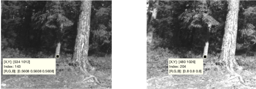
Figure 4.9: Left and right stereo image of the same scene. Corresponding points are marked manually in Matlab.
