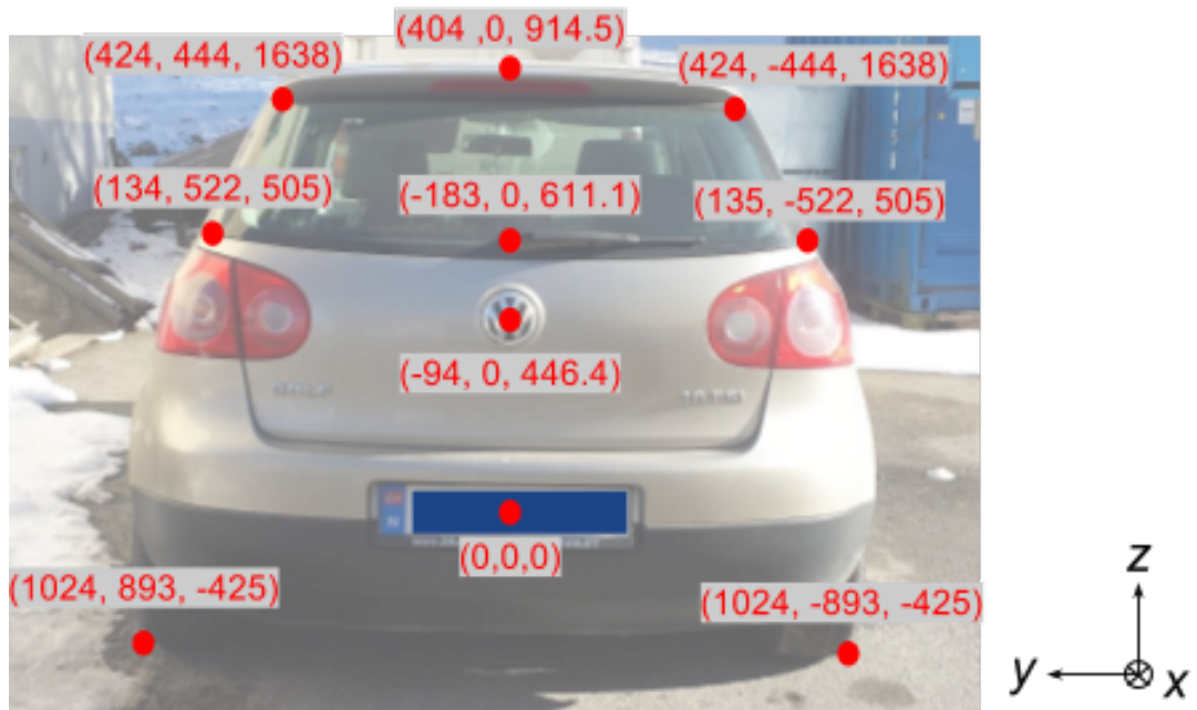
Figure 4.20: 3D model of the Golf. All feature points are relative the centre of the license plate. Units in millimetres.
