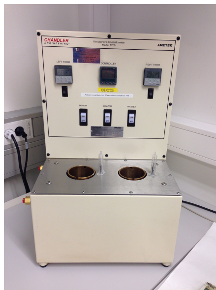
Figure 17: Atmospheric consistometer used to condition a cement slurry.
