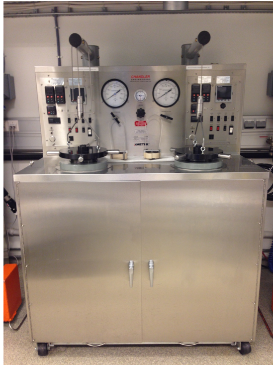
Figure 15: Pressurised consistometer used to determine thickening time of a cement slurry.
