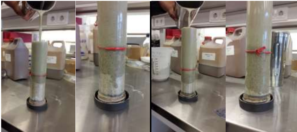
Figure3.26: Left: Diffusion for reference fluid, 72°F left t = 0 min, right t= 30min Right: Total intrusion for 0,3g nano silica fluid, 72°F left, t = 0 min, right, t = 2min
