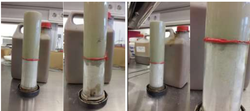
Figure 3.25: Left : Diffusion for the reference fluid in low porosity sand pack, 72°F, left t = 0min, right = 150min Right: Repulsion for the 0,3g nano silica fluid in low porosity sand pack, 72°F left t = 0 min, right t= 60min
