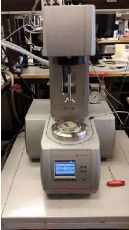
Figure 3.22: Illustration of Anton Paar MCR 301 Rheometer
