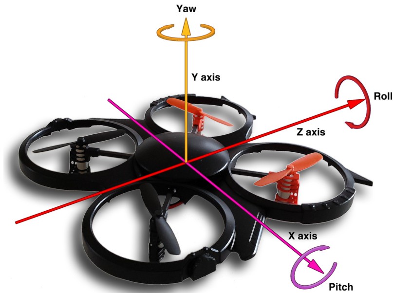
Figure 3.7: The pitch, yaw and roll that define an arbitrary rotation of a drone.
