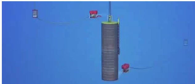
Fig. 4.2 Lowering of suction anchor to seabed. ROV's are employed to monitor the operation
