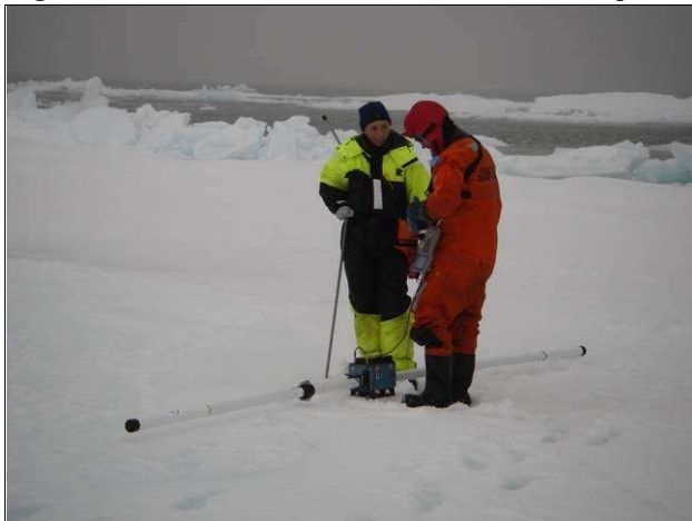
Fig. 2.3: Use of the Geonics EM31 for indirect ice plus snow thickness measurements.
