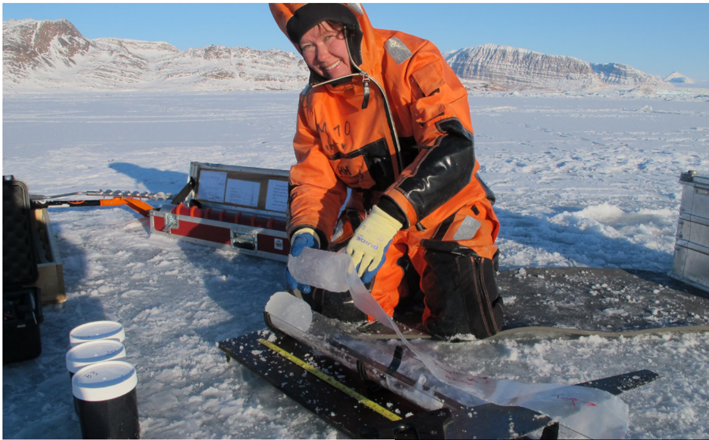
Sea ice sampling using an ice corer. Photo: Melissa Chierici, Institute of Marine Research
