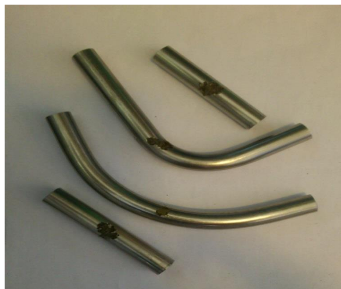
Figure 26: Crevices on Duplex Materials
