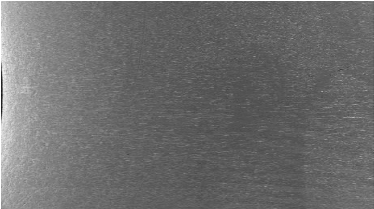
Image: Duplex Smaller Bend at after G48 Test at 30°C
