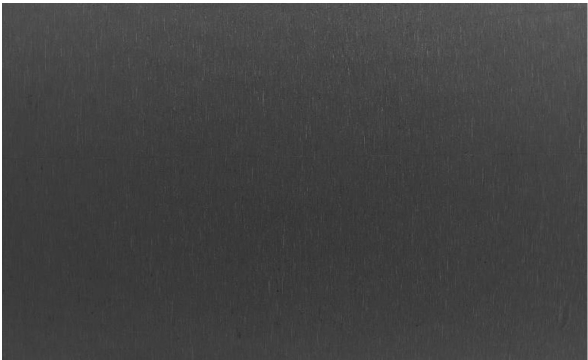
Image: Duplex Large Straight at after G48 Test at 30°C
