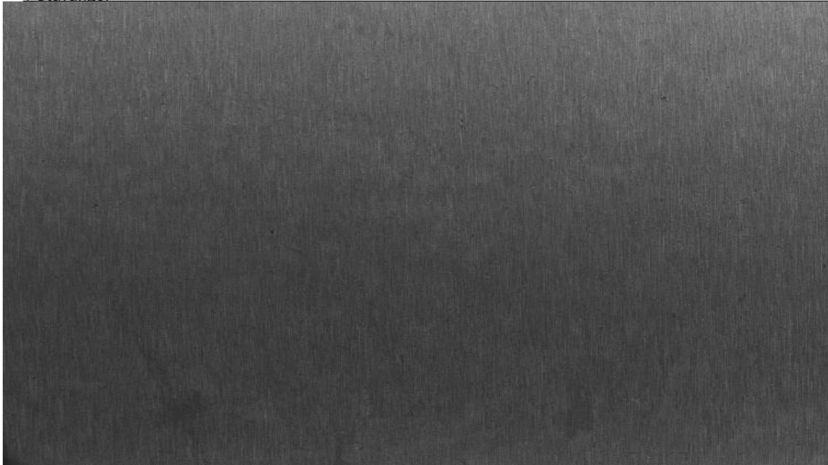
Image: Duplex Large Straight after G48 Test at 22°C
