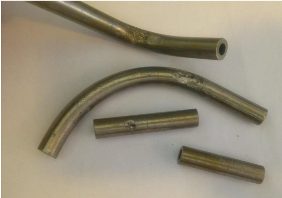
Figure 42: Super Duplex specimens after G48 Test at 60°C
