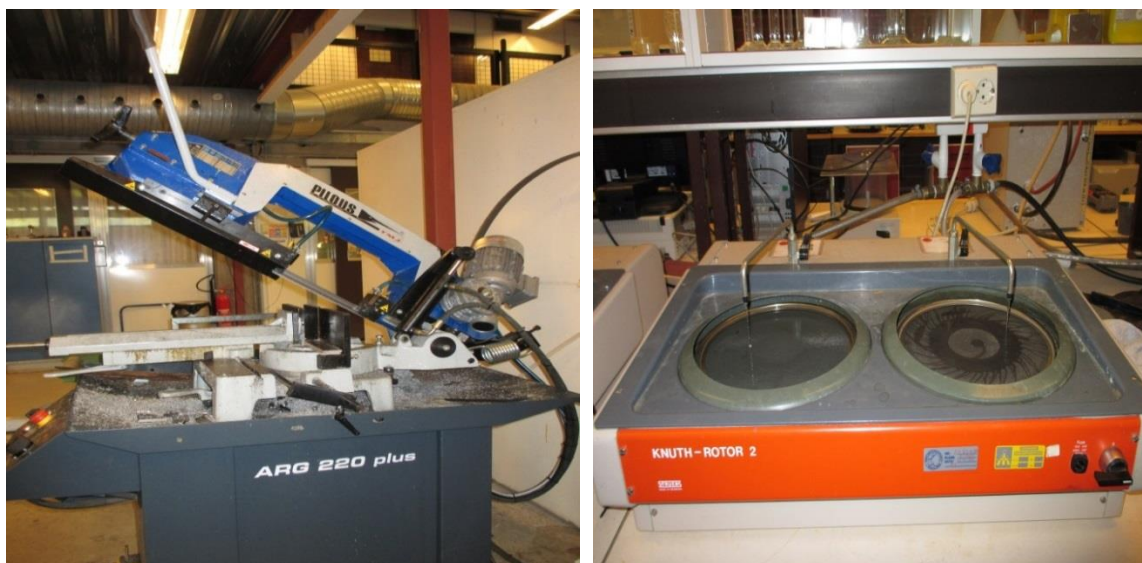
Figure 13: Mechanical Saw (left) and 120-Grit Abrasive Paper (Right)
