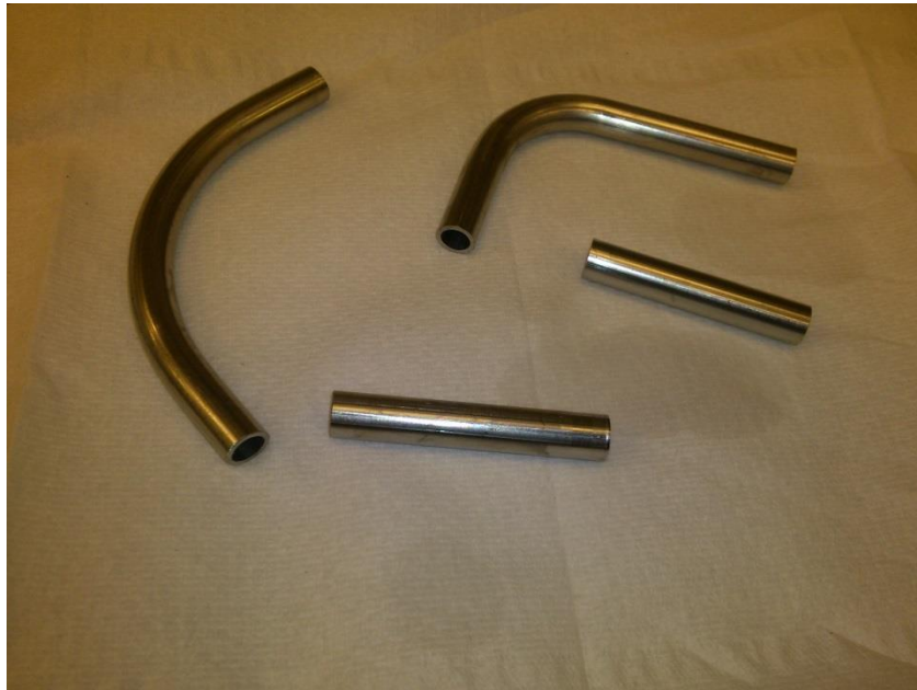
Figure 14: Duplex UNS S32205 Specimen ready for Testing ASTM G48
