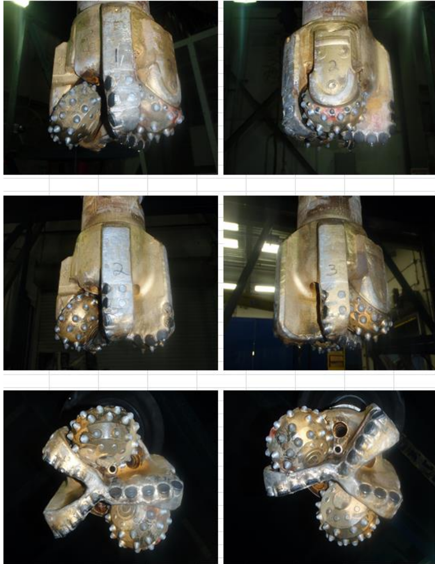
Figure 51 9.5 inch Kymera photos after the test was conducted
