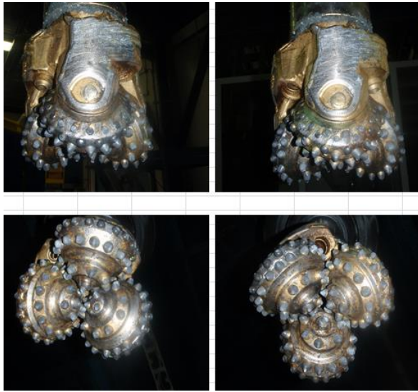
Figure 57 9.5 inch TCI Photos after the test has been conducted
