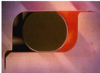
Figure 22 The seal function is to separate the cone grease from the oil
