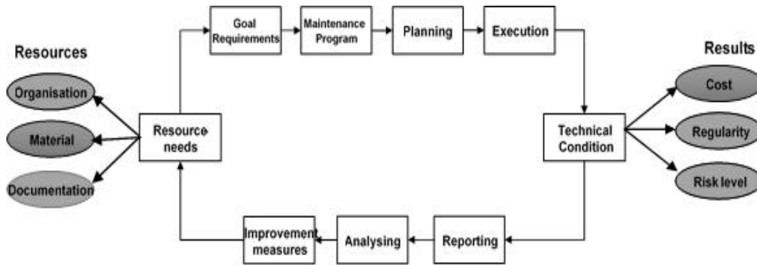
Figure 8: Maintenance Model Source: (Norwegian and Directorate, 1998)
