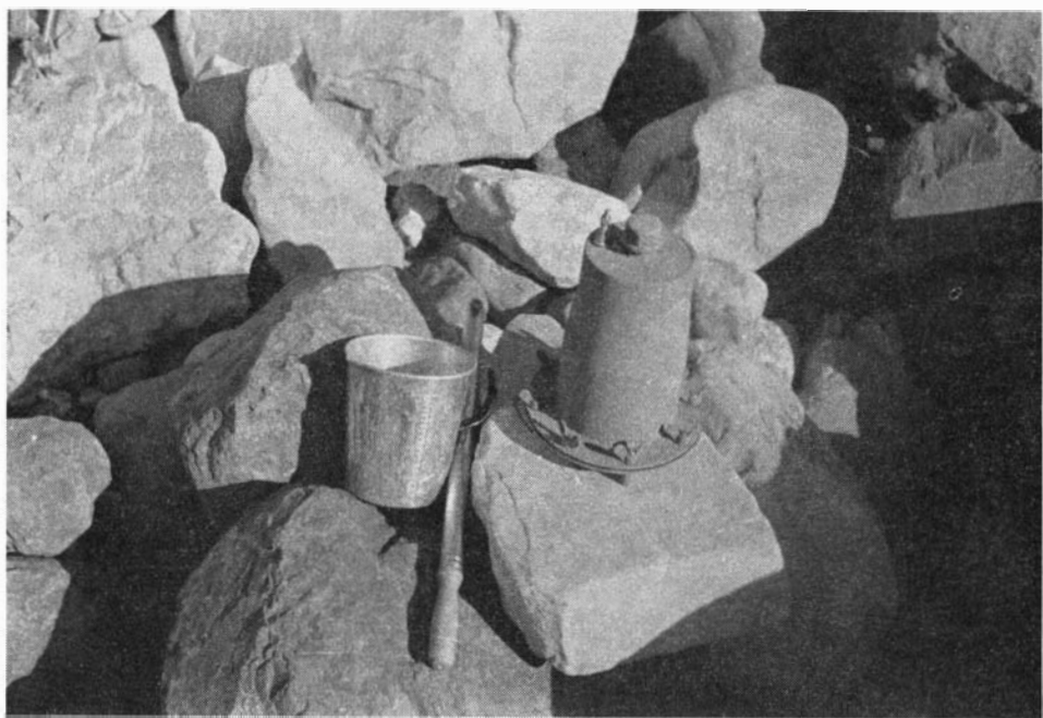
Fig. 40. The photo shows the equipment which was used for the measurements of sediment load. The filter lies against a perforated plate, screw fast to the holder to the right in the picture. After the holder becomes full of water, air is pumped in to speed up the filtering.
